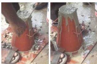
**Fig. 1. Subsidence test in progress**
