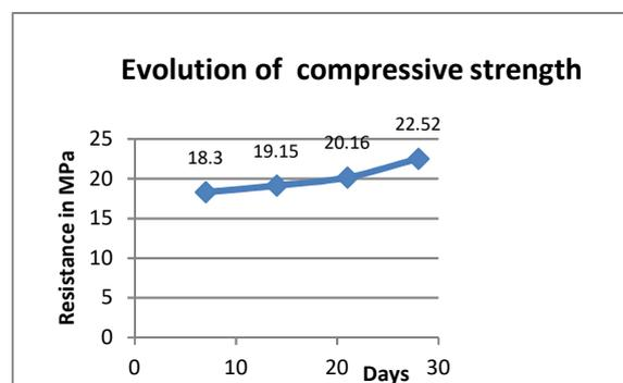
The breaking stress of the concrete used for the construction of the beams is :  $f_{c28} = 22.52$  MPa
