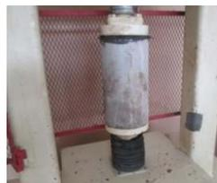
**Fig. 2. Start of compression test on hydraulic press**
