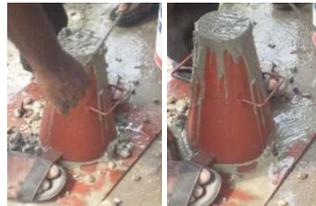
**Fig. 1. Subsidence test in progress**
