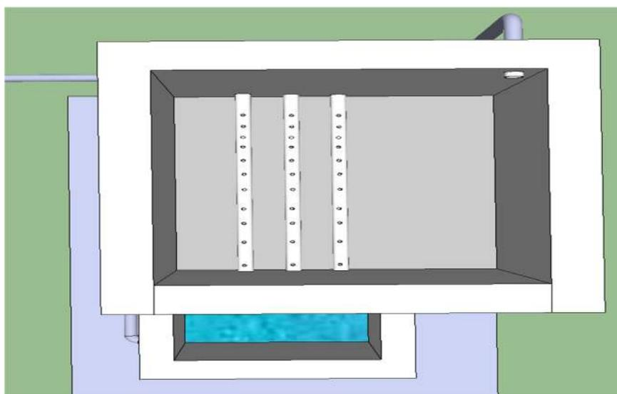
**Fig. 7. Top View of Modified Rapid Sand Filter**
