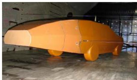
**Fig. 8. SUV model with rear fairing [31]**
