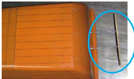
**Fig. 7. SUV model with rear screen [31]**
