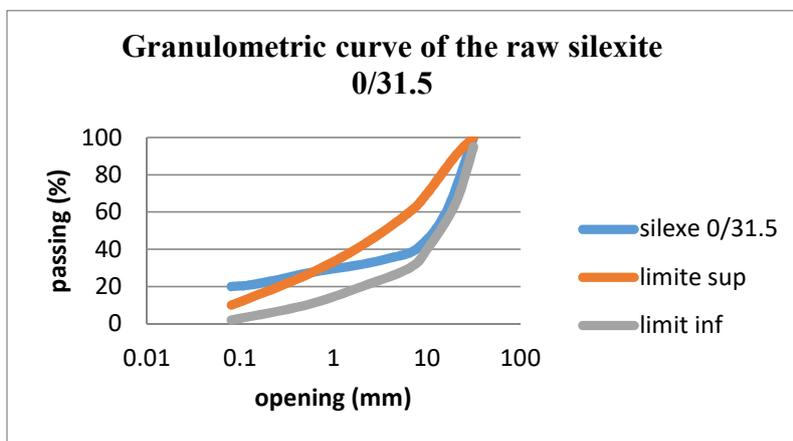
Fig. 3. Particle size of the crushed bass 0/31.5
