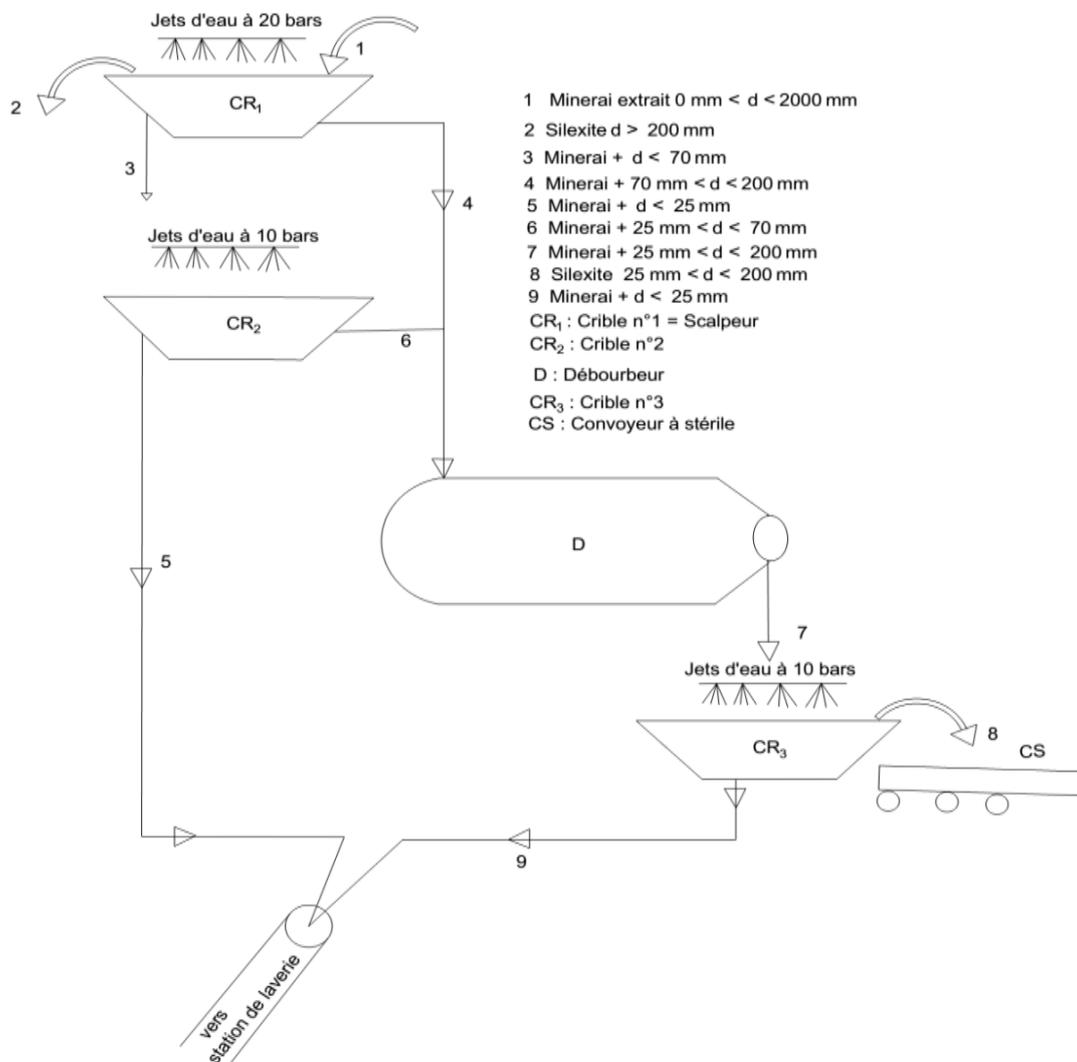
Fig. 1. Diagram of the clearing operation
