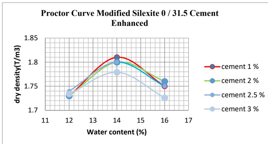
Fig. 9. Proctor curve modified with 0 / 31.5 silixite with cement improvement
