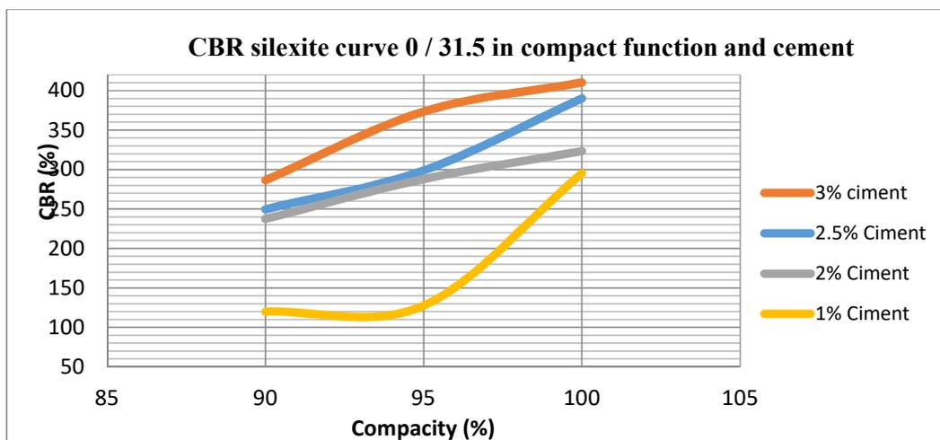
Fig. 14. CBR silixite curve 0 / 31.5 in compact function and cement
