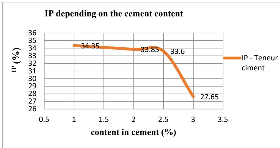
Fig. 8. IP by Cement Content
