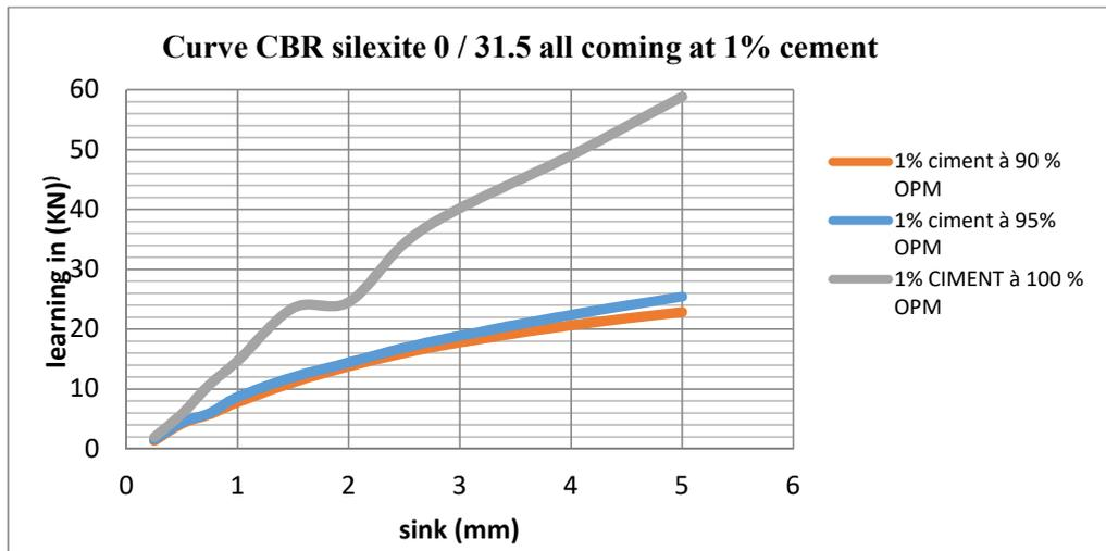
Fig. 10. Curve CBR silixite 0 / 31.5 at 1% cement
