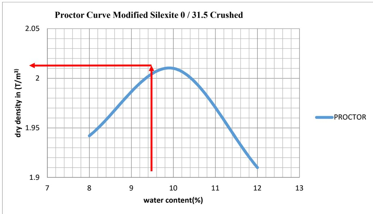
Fig. 17. Proctor Curve Modified Silexite 0 / 31.5 Crushed
