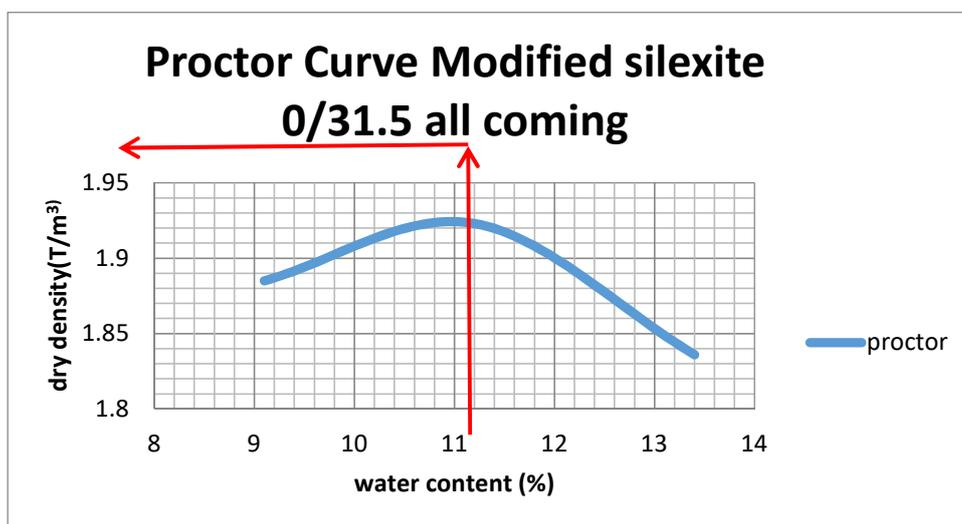
*Fig. 6. Modified Proctor Curve Silixite 0 / 31.5 Raw*
