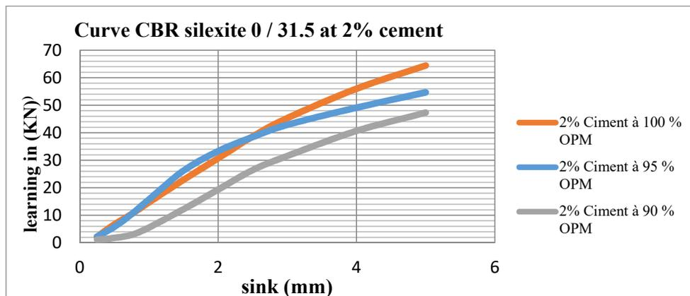
Fig. 11. Curve CBR silixite 0 / 31.5 at 2% cement
