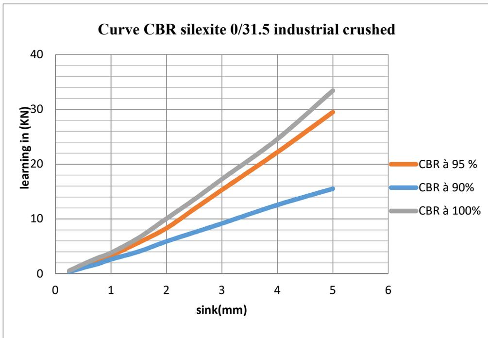
Fig. 18. Curved CBR curve 0 / 31.5 crushed industrial
