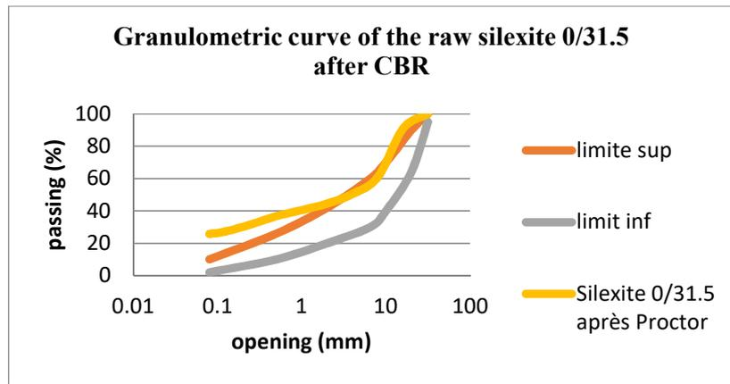
Fig. 4. Particle size of the crushed bass 0/31.5 after CBR.
