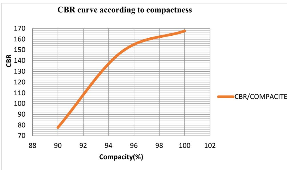
Fig. 19. CBR curve according to compactness
