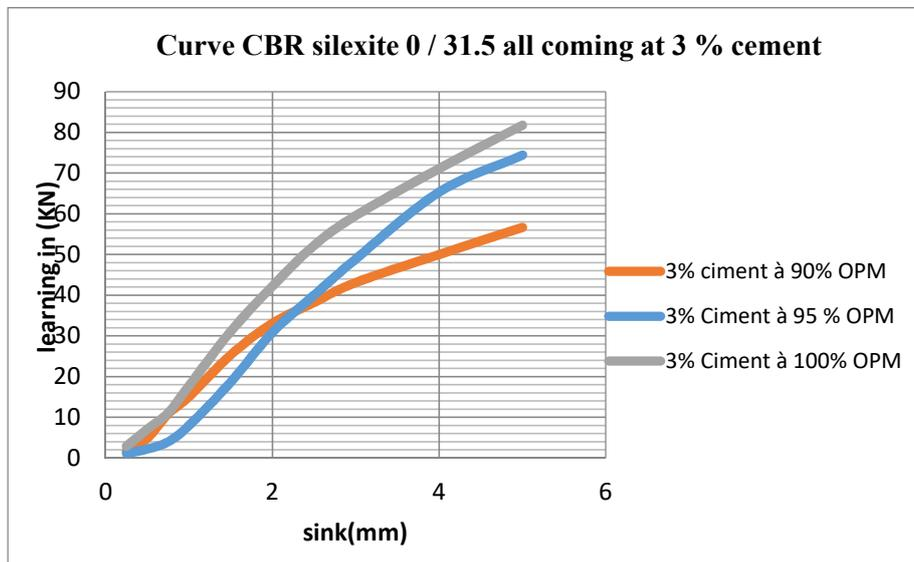
Fig. 13. Curve CBR silixite 0 / 31.5 all coming at 3 % cement
