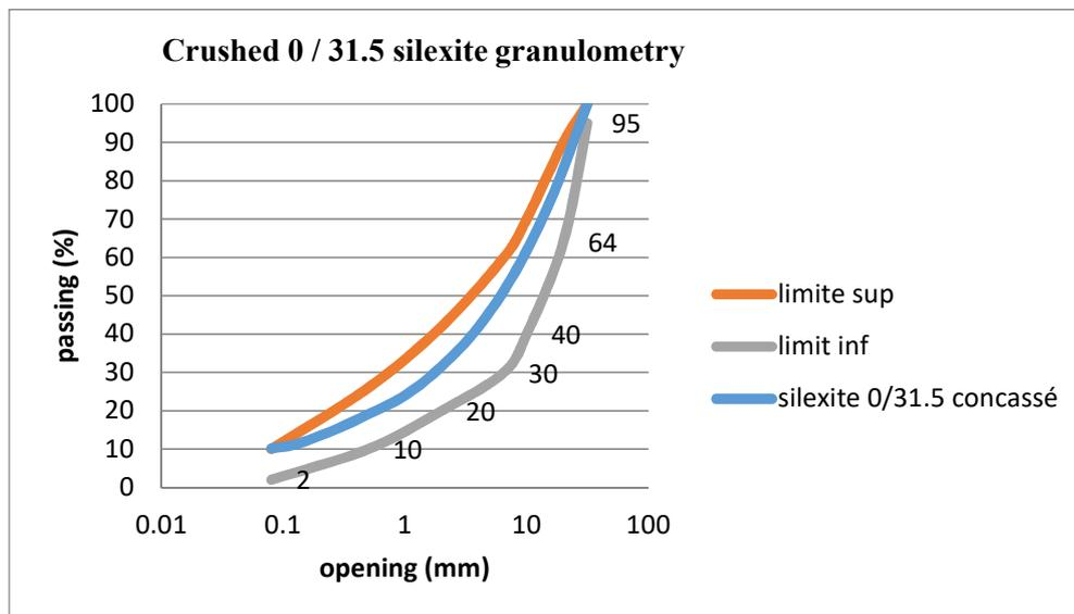
**Fig. 15. Industrial crushed particle size 0 / 31.5 according to the spindle**
