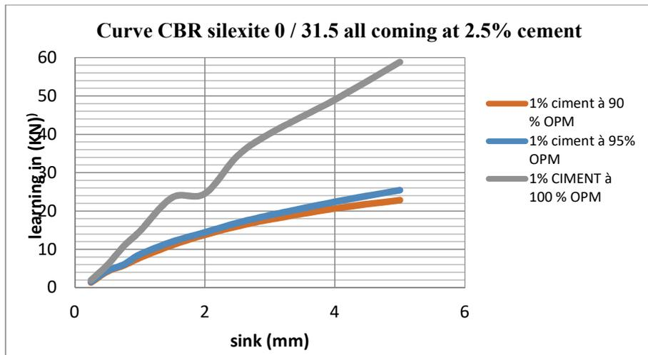
Fig. 12. Curve CBR silixite 0 / 31.5 all coming at 2.5% cement
