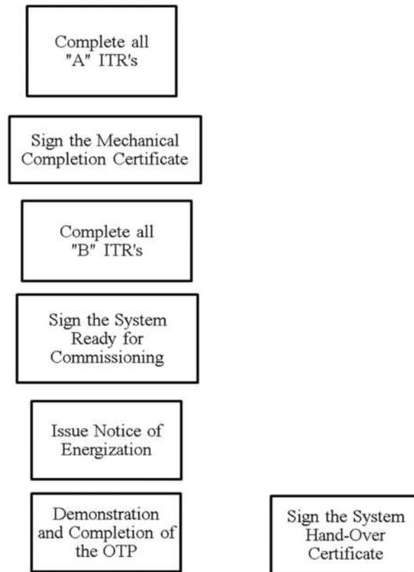
**Fig. 2. Mechanical Completion Flow for Commissioning**
