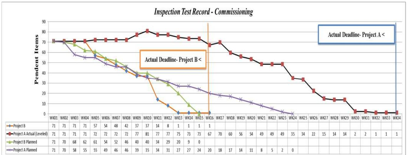
Fig. 11. Heating Medium System - Planned x Actual Curves for the Commissioning – Projects A and B.
