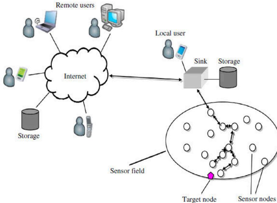
**Fig. 1. A Typical Wireless Sensor Network**
