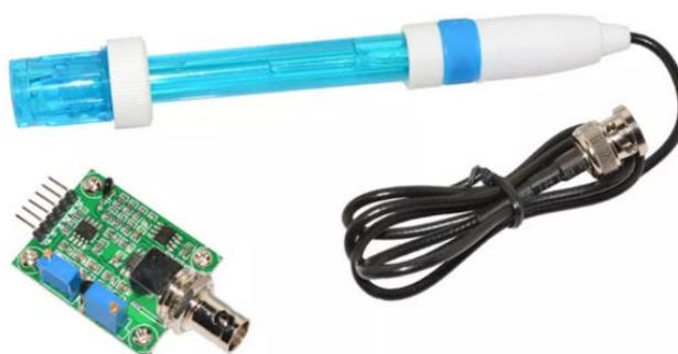
**Fig. 4. pH sensor with probe**
