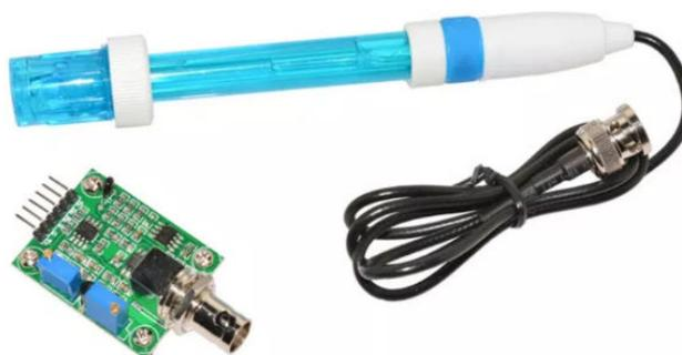
**Fig. 4. pH sensor with probe**
