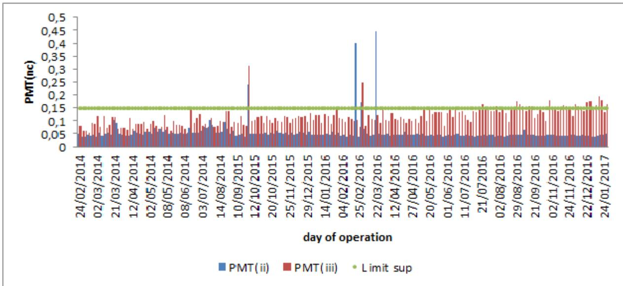
Fig. 2. Evolution of the PMT noise of the pellets in positions (ii) and (iii) according to the day of operation of the reader
