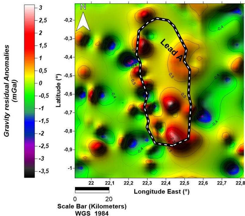
**Fig. 7. Gravity residual anomalies map of lead A**
