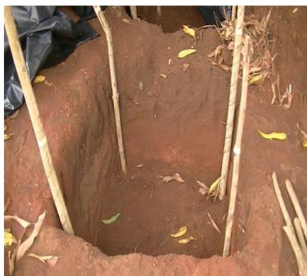
*Photo 1 a: 0.5m<sup>3</sup> pit delimited by four rods*
