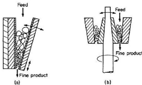
Fig.1.2.3 a) Jaw Crusher b) Gyratory crusher
