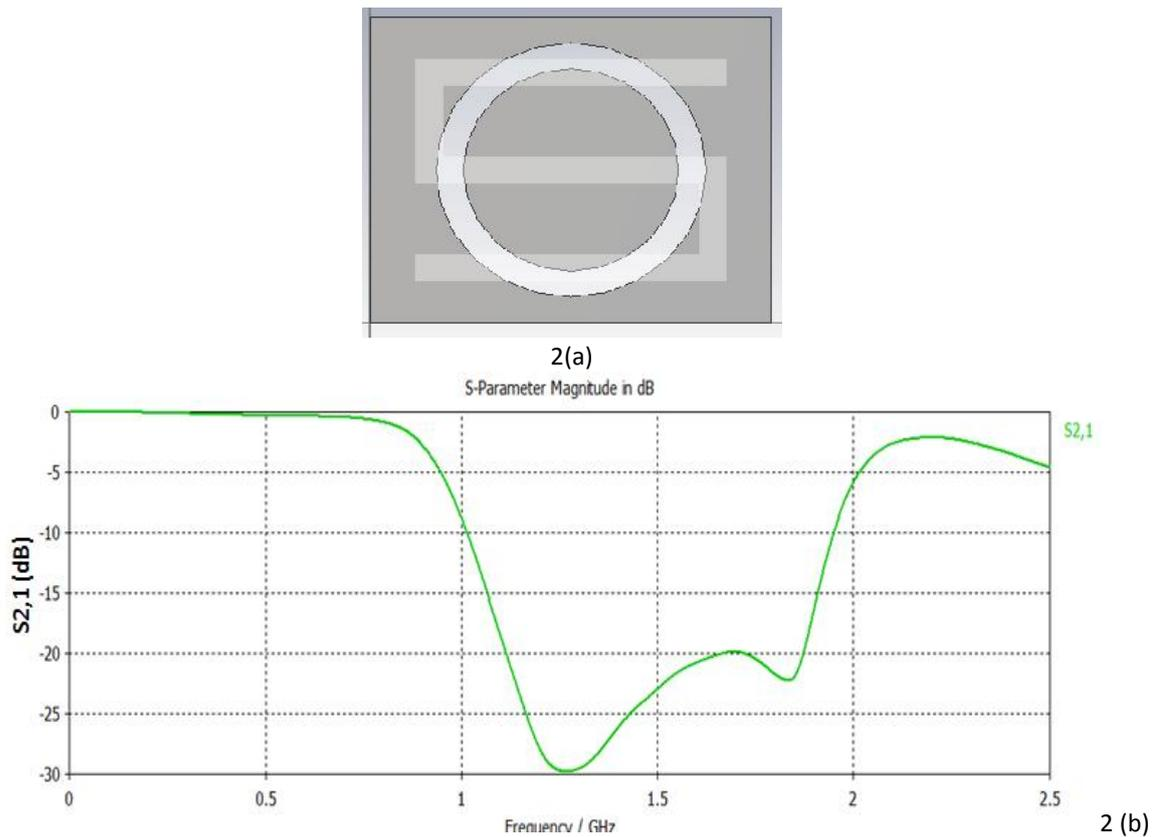
Fig.2 Schematic of: 2(a) S-shaped MLIN structure with ring etched in ground Plane, 2(b) Simulated S-parameter of structure.
