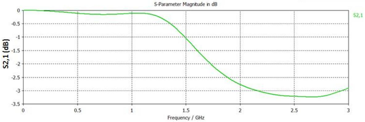
Fig.1(c) Schematic of Simulated S-parameter of S-shaped MLIN.
