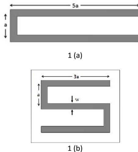
Fig. 1. Schematic of: 1(a) U-shaped MLIN and 1(b) S-shaped MLIN
