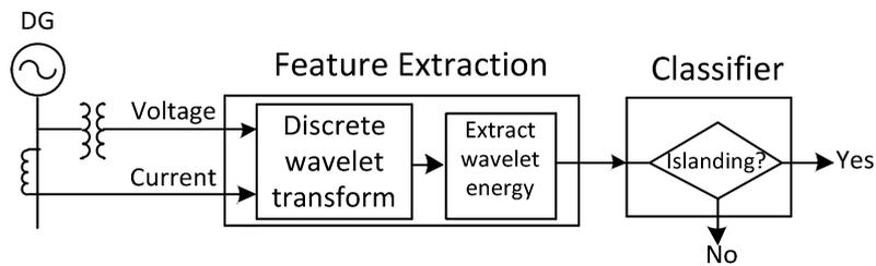
Fig.6 basic model of wavelet transform-based method
