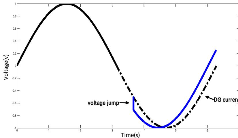
Fig5: Phase jump method Operation
