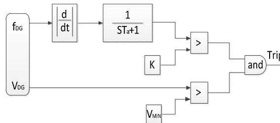
Fig3: ROCOF relay model
