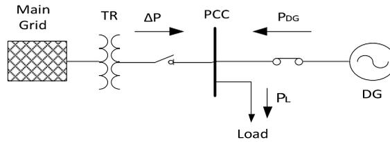
Fig2: System representation for anti-islanding methods
