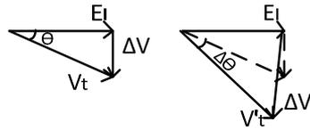
Fig 4: DG terminal voltage vector shift
