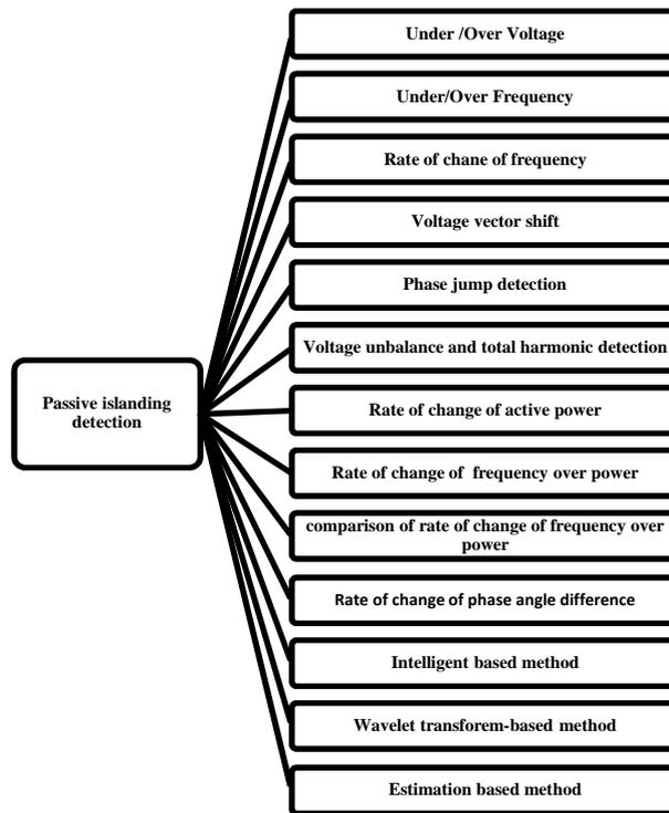
Fig7. Classification of passive islanding detection method
