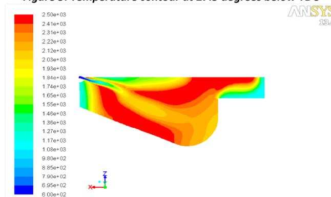
Figure 6: Temperature contour at 30 degrees below TDC
