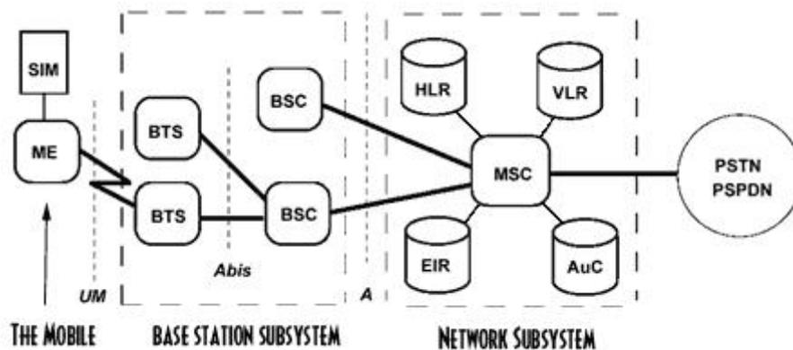
Figure 1 - Logical View of a Mobile Computing System
