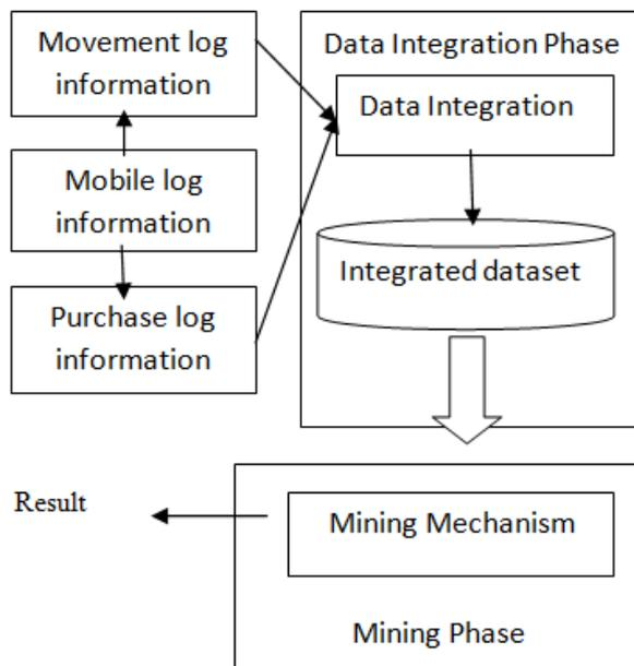
Fig. 2. System architecture for mobile log process
