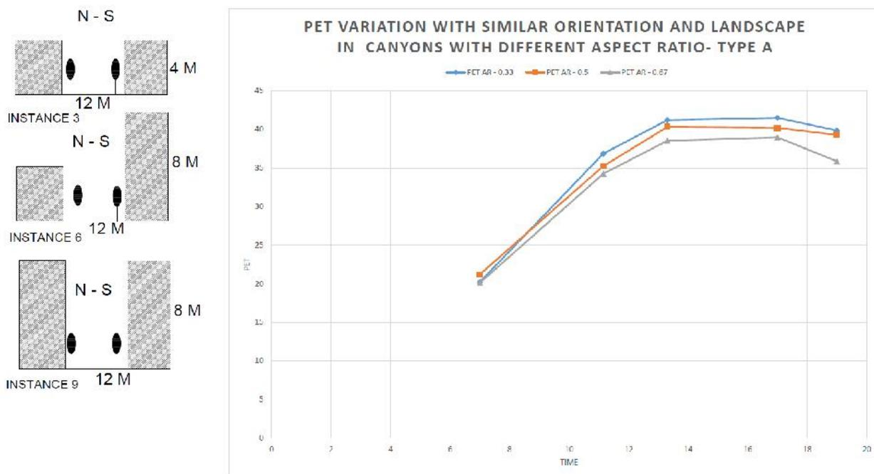
Fig 14: PET variation with alteration in Aspect Ratio – TYPE A street
