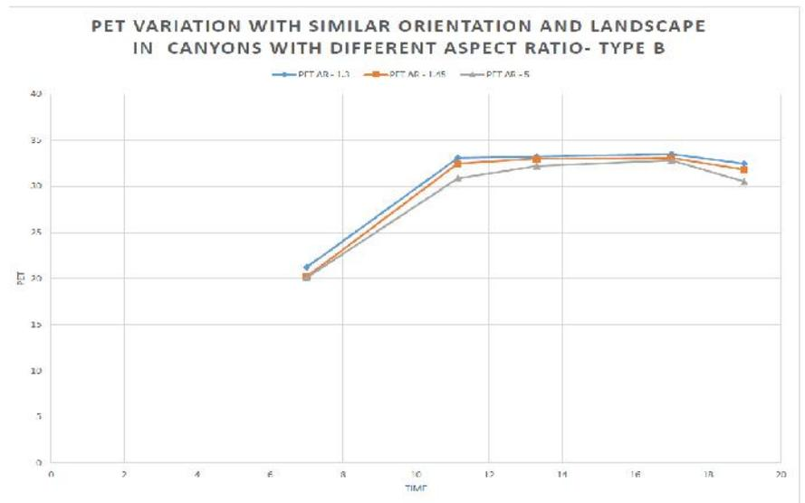
Fig 15: PET variation with alteration in Aspect Ratio – Type B street
