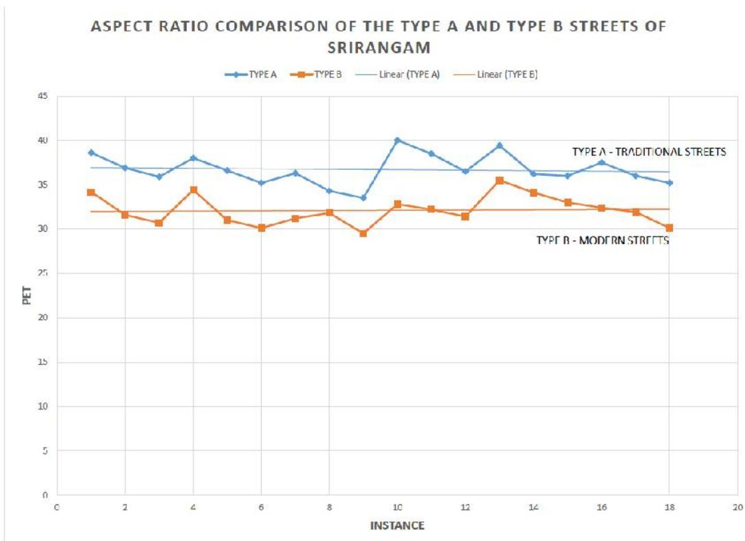
Fig 16: PET value comparison between TYPE A & TYPE B streets.
