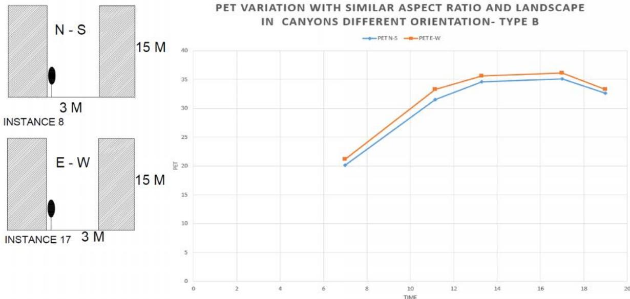
Fig 13: PET variation with alteration in orientation – Type B street
