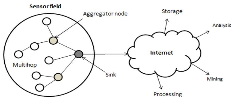
Fig.1. Architecture of Wireless Sensor Network
