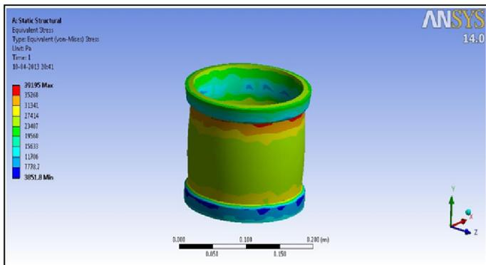
Figure 12: stresses induced in the glass structure
