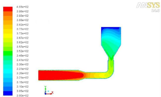
Figure 9: Temperature variation at velocity = 8 m/sec
