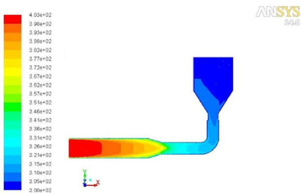
Figure 8: Temperature variation at velocity = 2 m/sec
