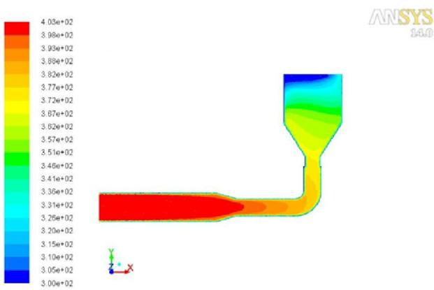
Figure 10: Temperature variation at velocity = 15 m/sec
