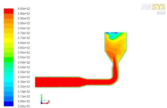
Figure 11: Temperature variation at velocity = 20 m/sec
