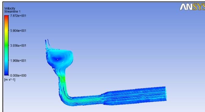
Figure 13: Flow happening in the Fluidised Bed Dryer
