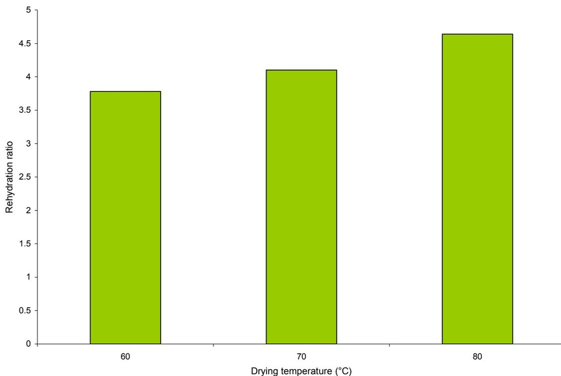
**Fig. 4.** Effect of drying temperature on rehydration ratio of the dried mango slices.
