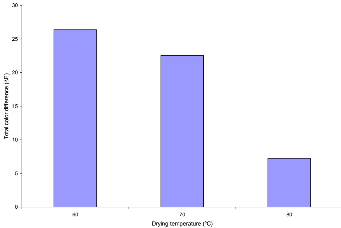
Fig. 3. Effect of drying temperature on total color change (ΔE)
