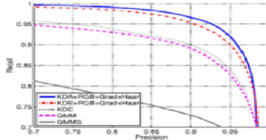
**Fig. 4. PR curves for different density estimations**
