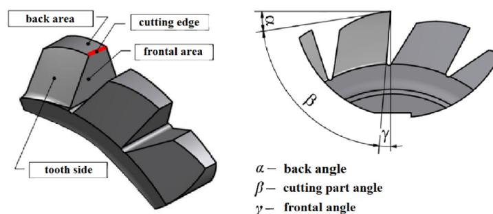
Fig. 6. Description of the hob gearing
