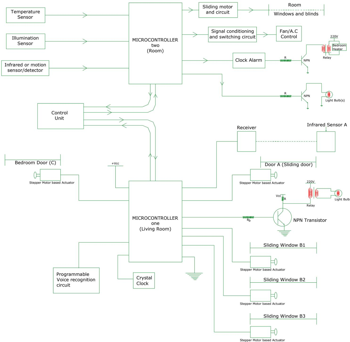
**Fig. 7. A Microcontroller base BAS design**
