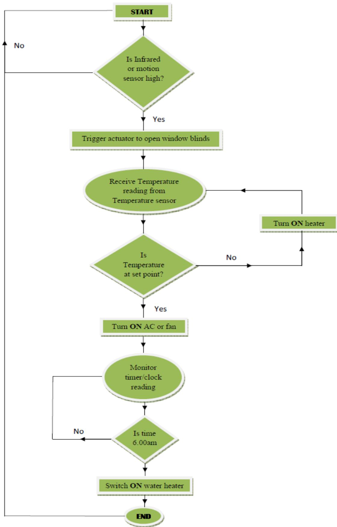
Fig. 4. Flow diagram showing the operation of the microcontroller
