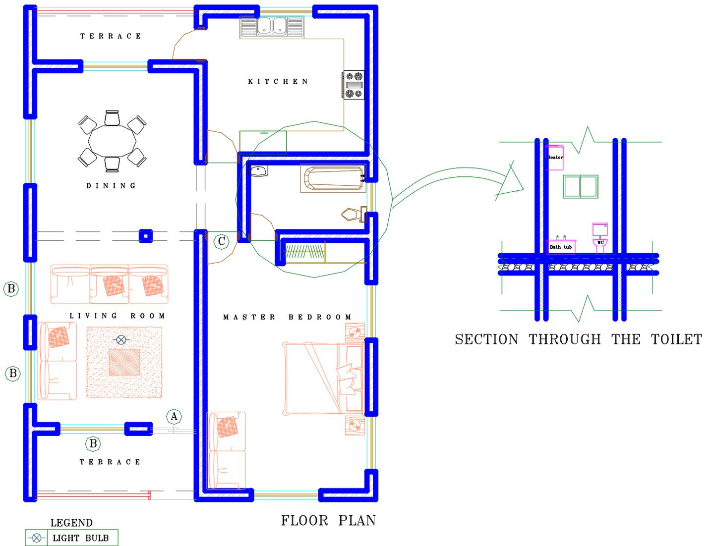
Fig. 5. Floor plan of the proposed building
