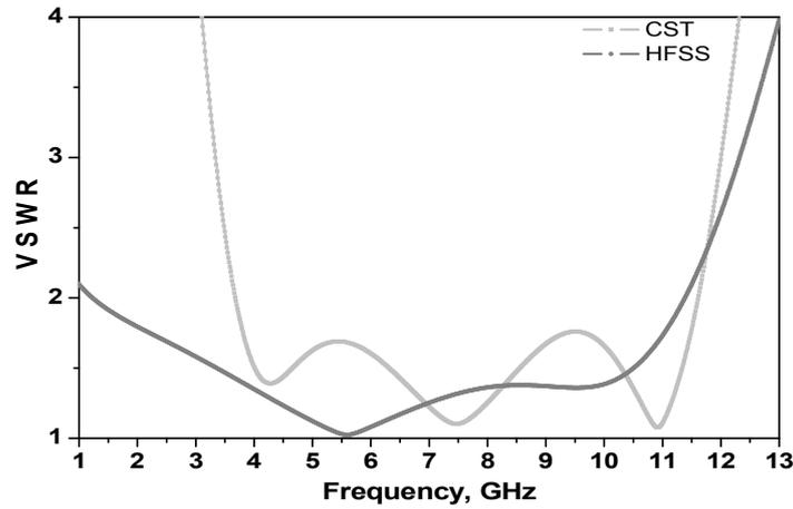
Fig. 3. Comparison between the simulated VSWR for the microstrip square antennas with HFSS and CST
