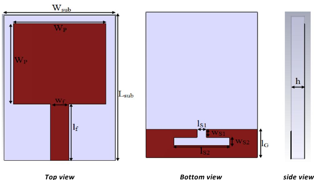
Fig. 1. Geometry of proposed antenna with inverted T-shaped notch
