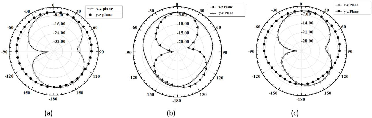
Fig. 4. E- and H-field patterns at different frequencies a-6GHz, b-7.38GHz and c-10.52GHz
