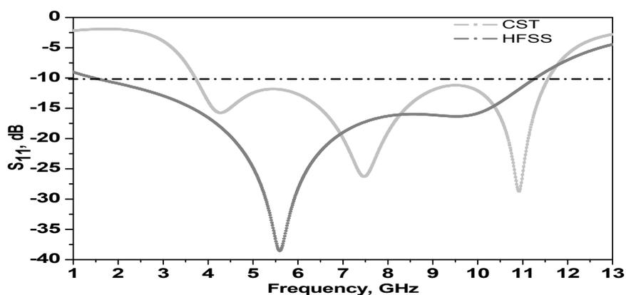
Fig. 2. Comparison between the simulated  $S_{11}$  for the microstrip square antennas with HFSS and CST
