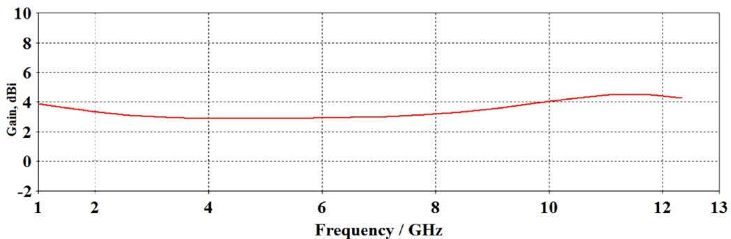
Fig. 5. Gain in dBi of square patch antennas against frequency
