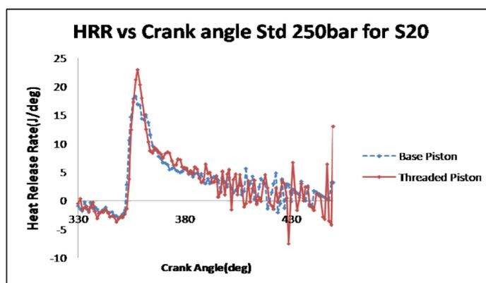
Fig.5. Heat release rate Vs Crank angle
