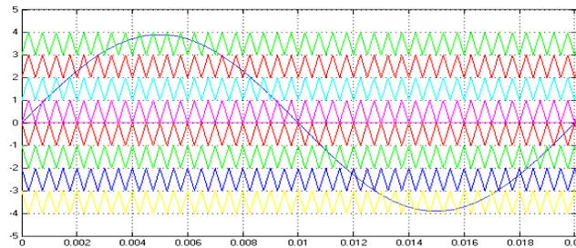
Fig.3. Carrier arrangement for Phase Opposition Disposition PWM strategy
