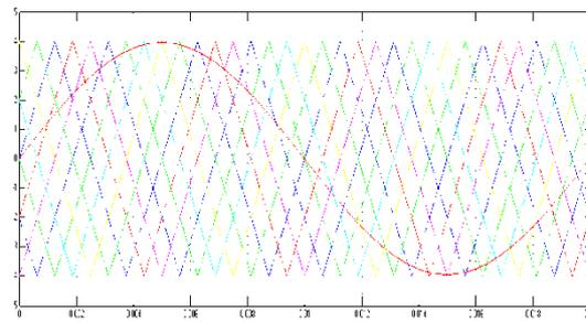
**Fig. 5. Carrier arrangement for Phase shift PWM strategy**
