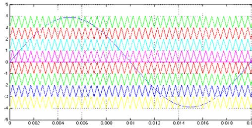
Fig. 2. Carrier arrangement for Phase Disposition PWM strategy
