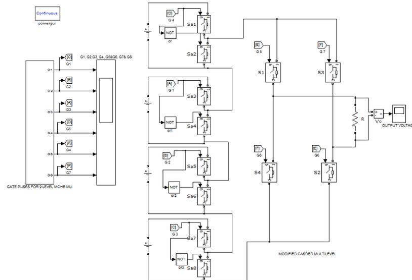
Fig. 6. Simulink Modeling of the Hybrid H-Bridge Multilevel Inverter
