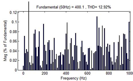
Fig. 16. FFT plot of 9-level Hybrid H Bridge MLI Using PSPWM Strategy
