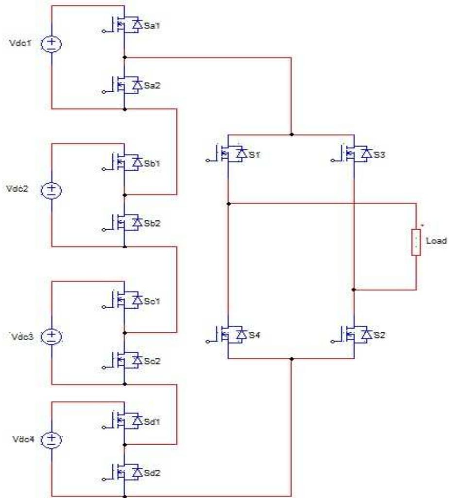
Fig. 1. 9-Level Hybrid H-Bridge Multilevel Inverter
