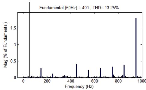
Fig. 12. FFT plot of Hybrid H Bridge MLI Using PDPWM Strategy
