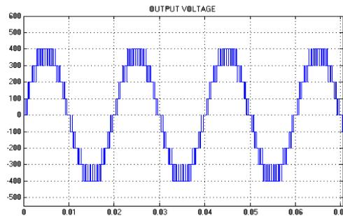
Fig .11. Simulated 9-level Output Voltage waveform of Hybrid H Bridge MLI Using PDPWM Strategy
