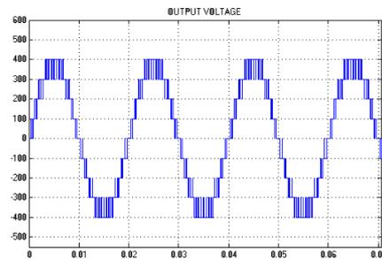
Fig .13. Simulated 9-level Output Voltage waveform of Hybrid H Bridge MLI Using APDPWM Strategy
