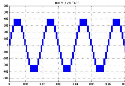
Fig. 15. Simulated 9-level Output Voltage waveform of Hybrid H Bridge MLI Using PSPWM Strategy
