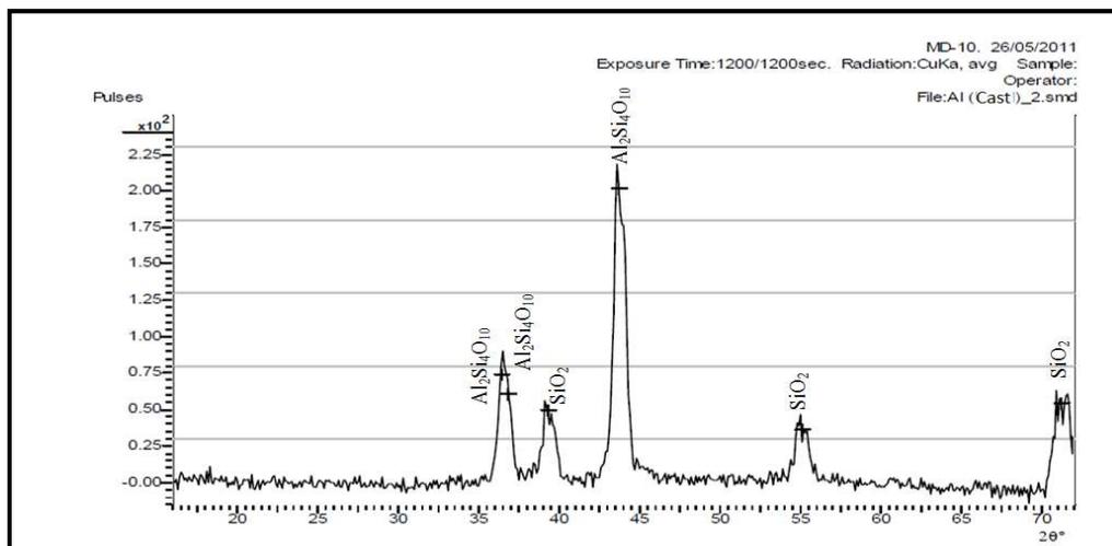
Figure 10: XRD analysis of cast aluminium alloy sample
