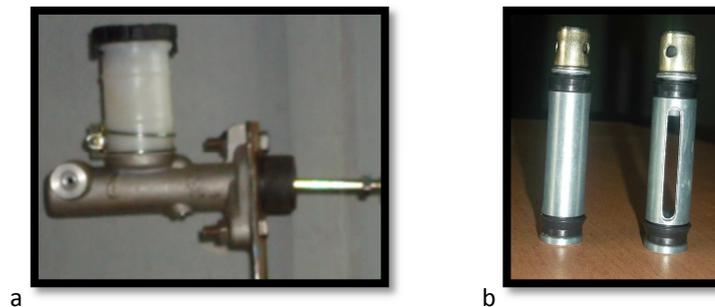
**Figure 2: Photographs showing of (a) as received master brake cylinder and (b) floating calliper**
