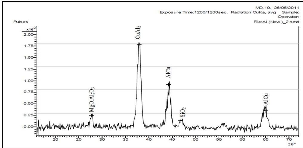
Figure 9: XRD analysis of As-received aluminium alloy sample
