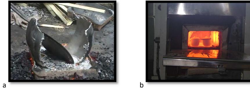
**Figure 1: Re-melting of aluminium in (a) an open earth-made furnace and (b) electric furnace.**
