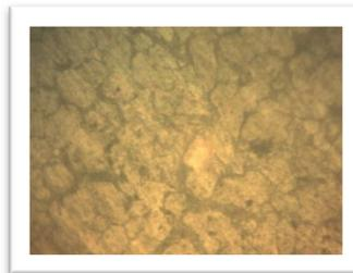
**Figure 5: Micro-structure of sample A under magnifications of x800**
