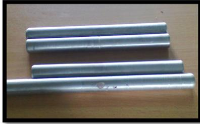
Figure 3: Turned aluminium alloy before slicing
