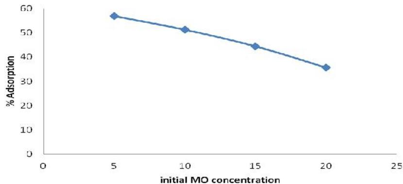
*Fig. 4. % adsorption Vs initail MO concentration*
