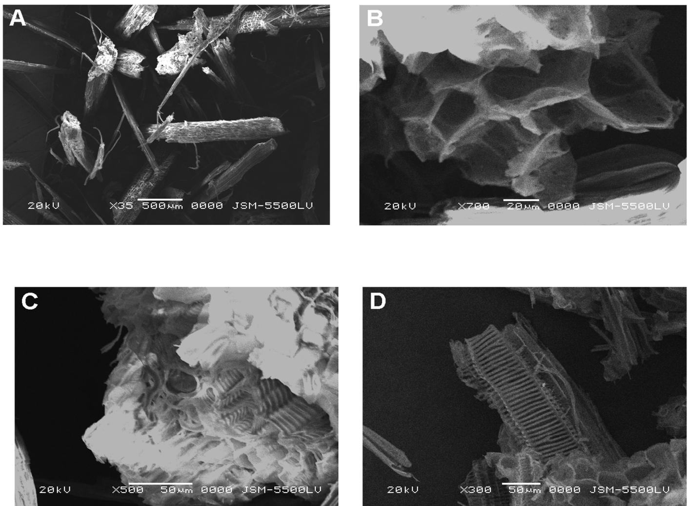
Figure.5: SEM of microphotograph of Date Palm rachis
