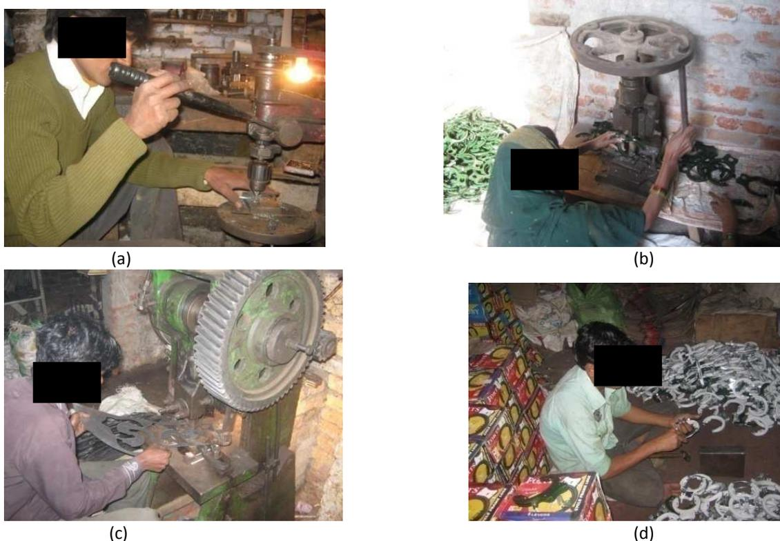
**Figure 1:- (a) Hand operated drilling machine, (b) Hand operated punching machine, (c) Foot operated punching machine, (d) Final inspection**
