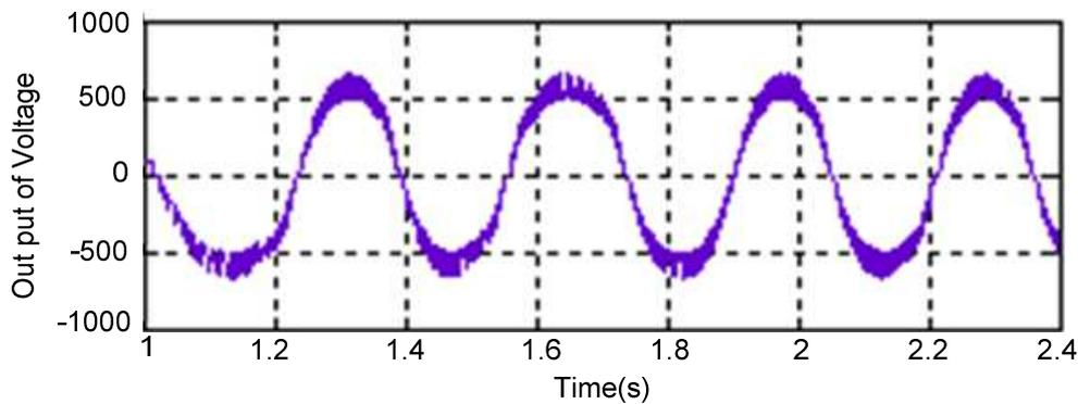
Fig 4: voltage waveform of phase A at the non-nominal state
