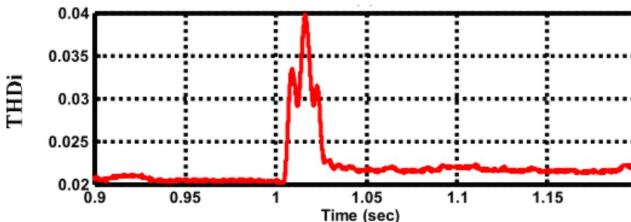
Fig 10: Changes of THD of current at nominal load on the islanding conditions
