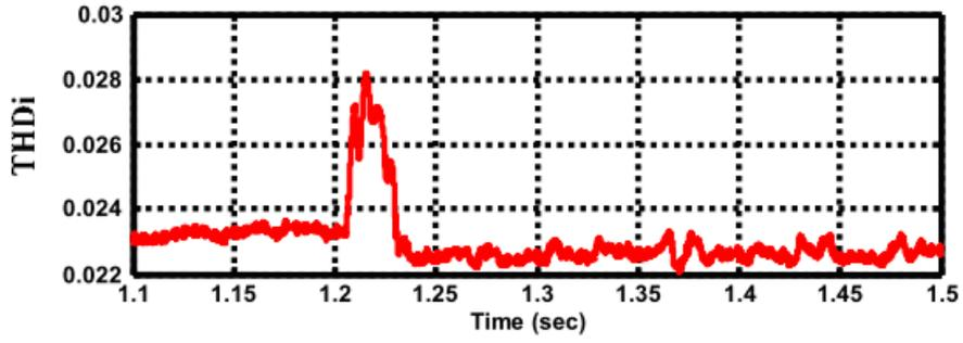
Fig 6: Changes of THD of current at non-nominal load on the islanding conditions
