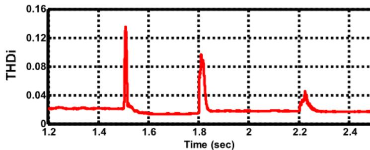
Fig 14: THD waveforms for current in the switching conditions
