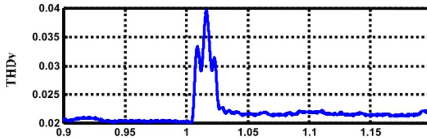
Fig 9: Changes of THD of voltage at nominal load on the islanding conditions
