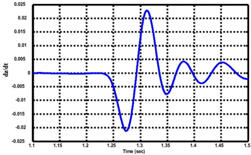
Fig 7: The rate of impedance changes in non-nominal conditions
