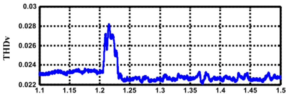
Fig 5: Changes of THD of voltage at non-nominal load on the islanding conditions
