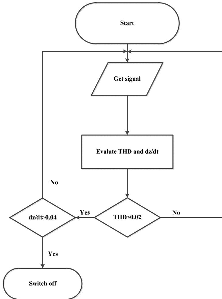
Fig 3: The flowchart of the proposed algorithm for detecting Islanding
