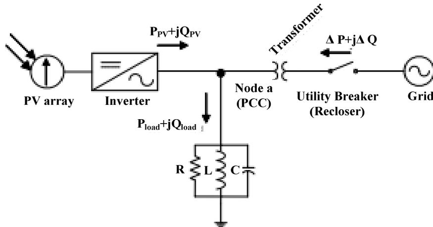
Fig 1: sketch of distributed generation system for detecting anti Islanding
