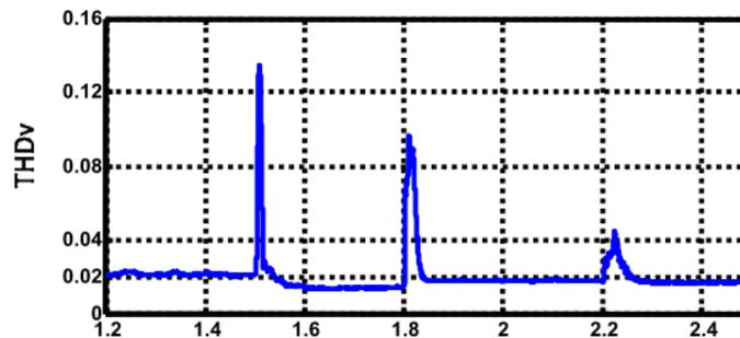
Fig 13: Changes of THD of voltage in islanding and switching state
