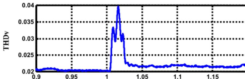
Fig 9: Changes of THD of voltage at nominal load on the islanding conditions
