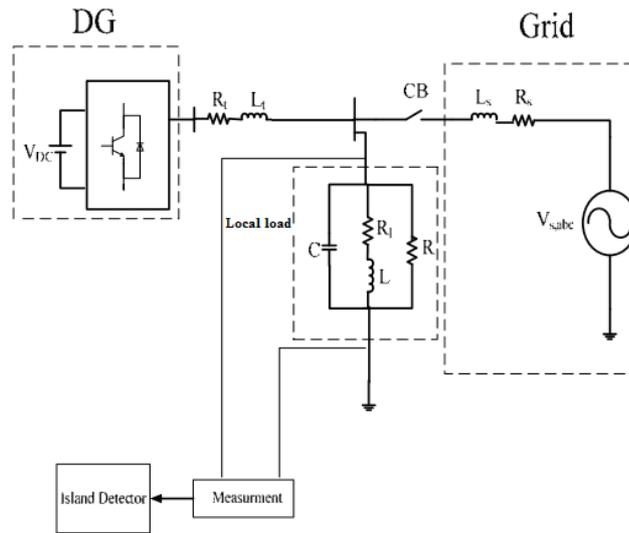
Fig 2: The power system being studied including distributed generation and network
