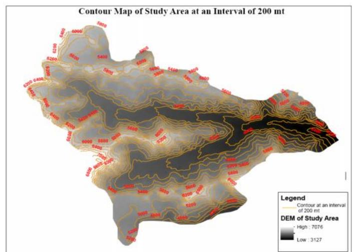
Fig4: Contour Map at an Interval of 200 mt using ASTER DEM
