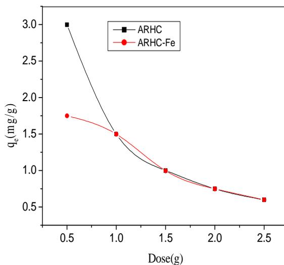
**Fig.5.** Effect of adsorbent dosage on the adsorption capacity of Methylene blue using ARHC and ARHC-Fe Conditions at  $C_0=30\text{ppm}$ .  $\text{pH} = 8$ ,  $t=120\text{ min}$ ,  $T= 25 \pm 2^\circ\text{C}$ .
