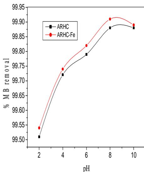
Fig.7. Effect of pH solution on the adsorption efficiency Methylene blue using treated ARHC and RHC-FeCl<sub>3</sub> at  $C_0=30$  ppm. ,  $W_{AC} = 1g$ ,  $t=120$  minutes and  $T= 25 \pm 2^\circ C$ .
