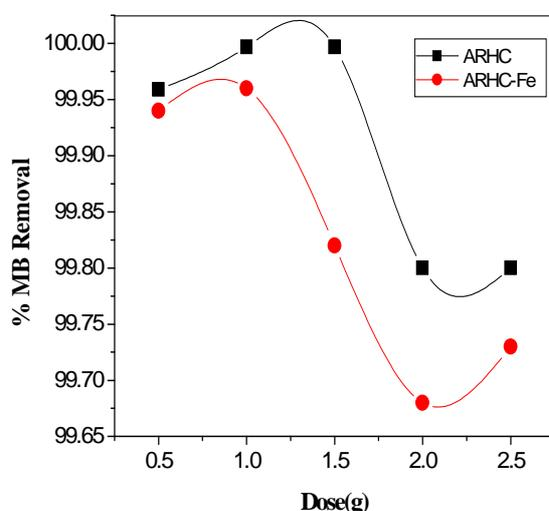
**Fig. 4:** Effect of adsorbent dosage on the adsorption efficiency of Methylene blue using ARHC and ARHC-Fe, at  $C_0=30\text{ppm}$ .  $\text{pH} = 8$ ,  $t=120\text{ min}$ ,  $T= 25 \pm 2^\circ\text{C}$ .
