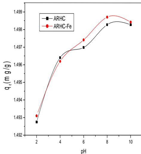
**Fig. 8. Effect of pH solution on the adsorption capacity Methylene blue using treated ARHC and RHC-FeCl<sub>3</sub> at Co=30 ppm. , W<sub>AC</sub> = 1g, t=120 minutes and T= 25±2°C.**
