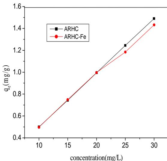
Fig.3. Effect of initial concentration on adsorption capacity of Methylene Blue using rice husk Carbon at 30 ppm. Conditions: pH = 8; t=120 minutes W<sub>AC</sub>= 1g and T= 25 ±2°C.
