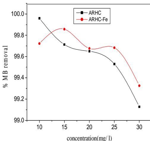
Fig.2. Effect of initial concentration the removal efficiency Methylene blue using treated rice husk carbon Conditions: pH = 8, t= 120 minutes, W<sub>AC</sub>= 1g, and T= 25 ±2°C.
