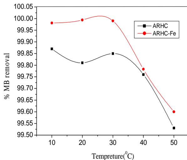
**Figure 9: Effect temperature on the adsorption efficiency Methylene blue using treated ARHC and ARHC-Fe at Co=30 ppm. , W<sub>AC</sub> = 1g, t=120 minutes and PH = 8.**
