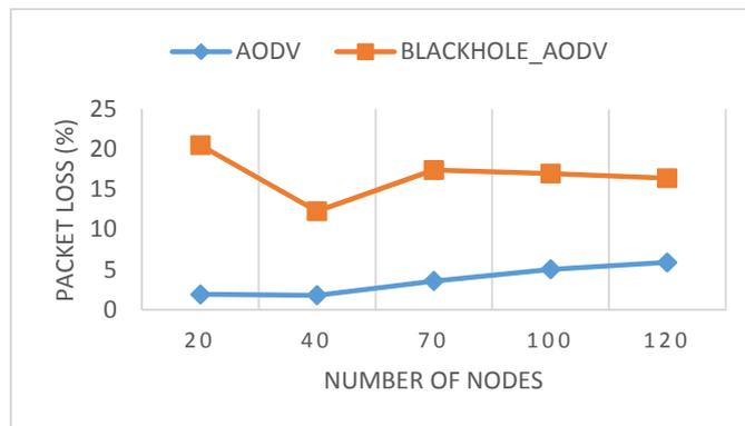
Figure 10 : Lost packets under the impact of a single malicious node in AODV
