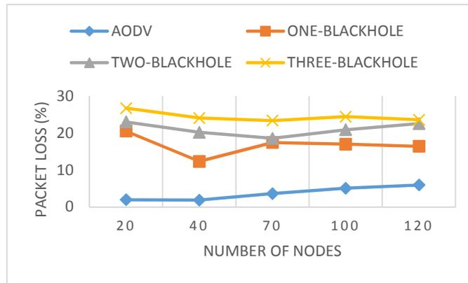
Figure 12 : Lost packets under the impact of three malicious nodes in AODV
