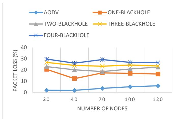
Figure 13 : Lost packets under the impact of four malicious nodes in AODV
