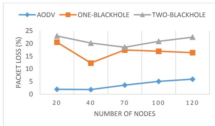
Figure 11 : Lost packets under the impact of two malicious nodes in AODV
