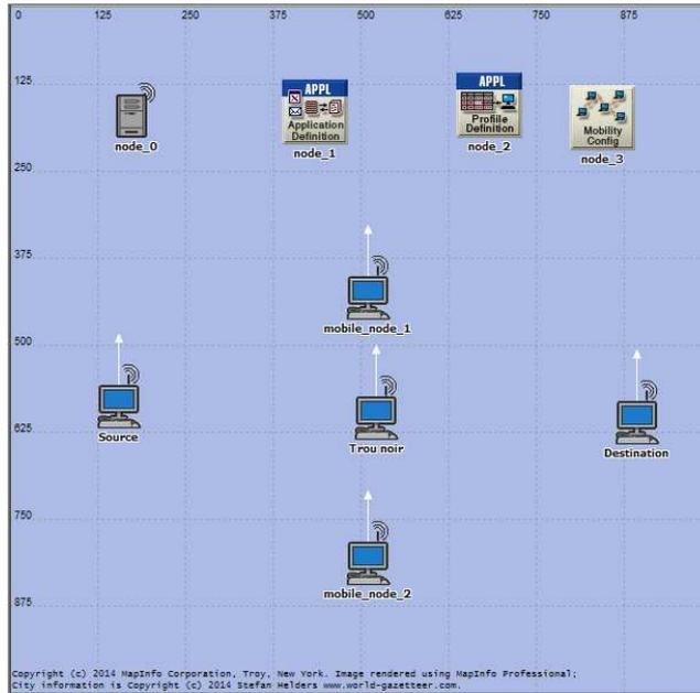
Figure 5 : Simulation environment with black hole.
