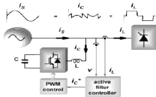
Fig 1: General Block Diagram For shunt a Active filter
