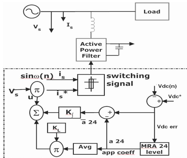
Fig. 7: Structure of wavelet Controller for APF
