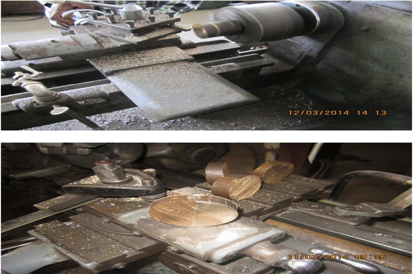
*Fig 2. Cutting and Turning of the Metal Brass*
