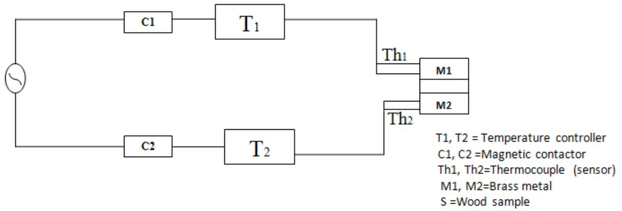
Fig 3 Block Diagram of the electrical set-up
