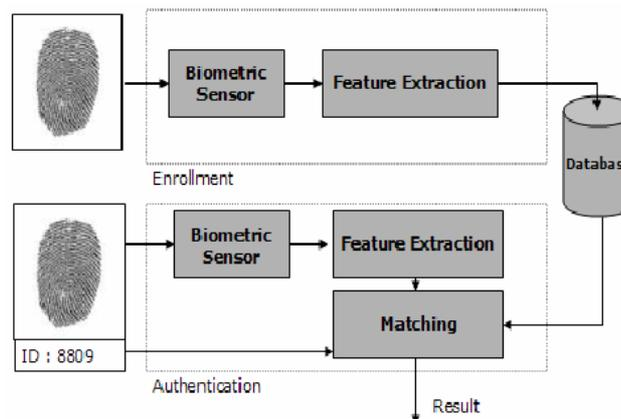
**Fig. 2. Block diagram of Fingerprint recognition system**
