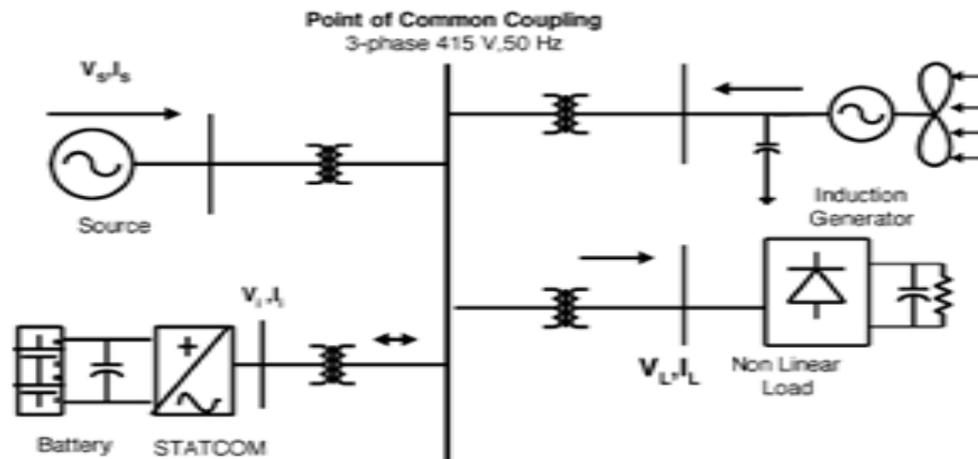
Fig. 1. Grid connected system for power quality improvement
