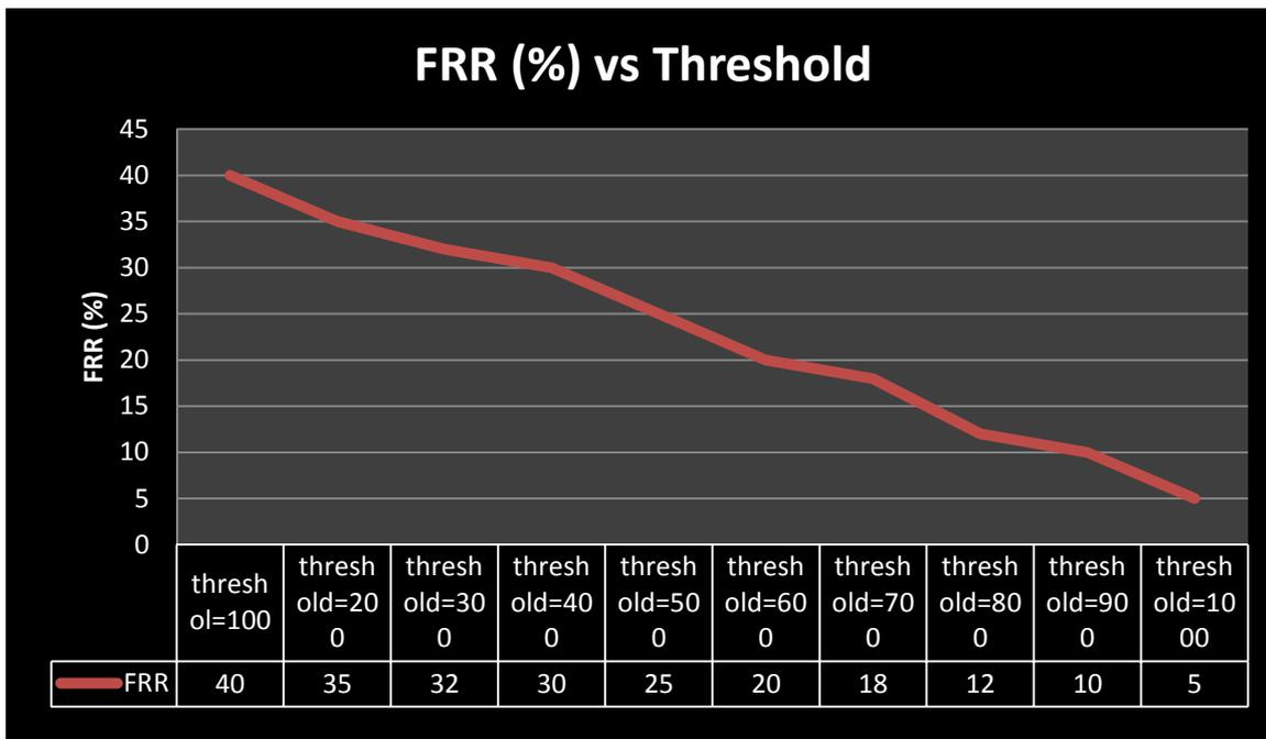
Figure 10 : False rejection rate Vs Threshold variance
