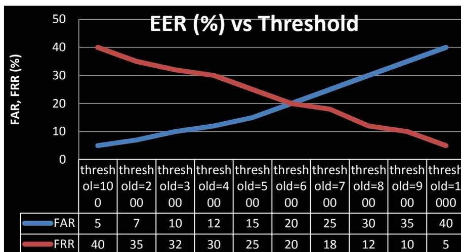
Figure 11: Equal Error Rate Vs Threshold variance
