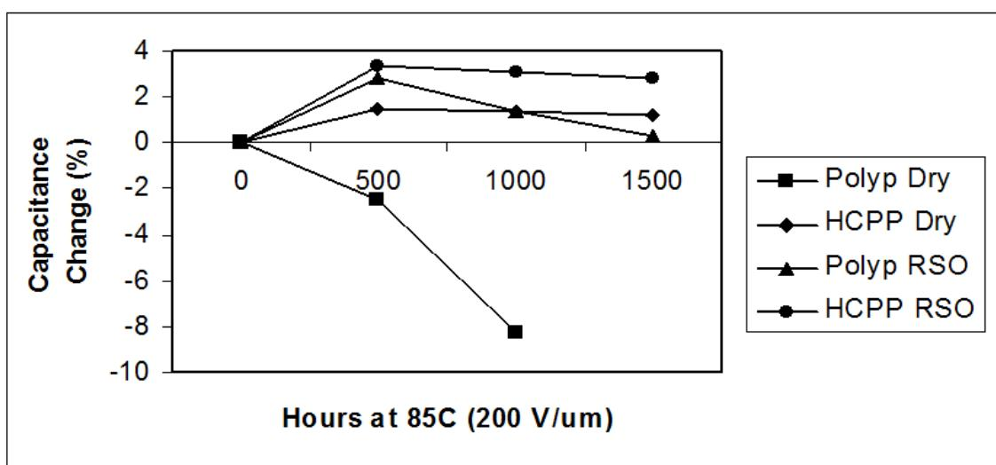
**Fig. 1. Performance of Five Micron Segmented Film In Capacitors**
