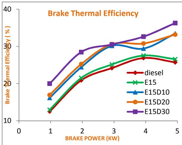
Fig 4: Brake power Vs BTE
