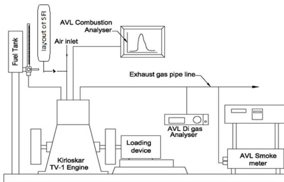
Figure 1: Layout of Experimental Setup with Secondary Fuel Injection (SFI).
