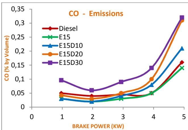
Fig 6: Brake power Vs CO Emissions.
