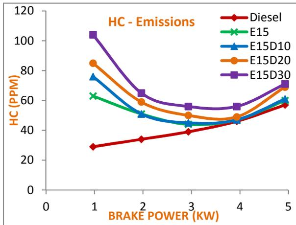
Fig 8: Brake power Vs HC Emissions
