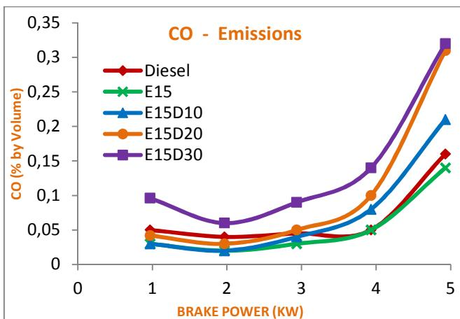
Fig 6: Brake power Vs CO Emissions.
