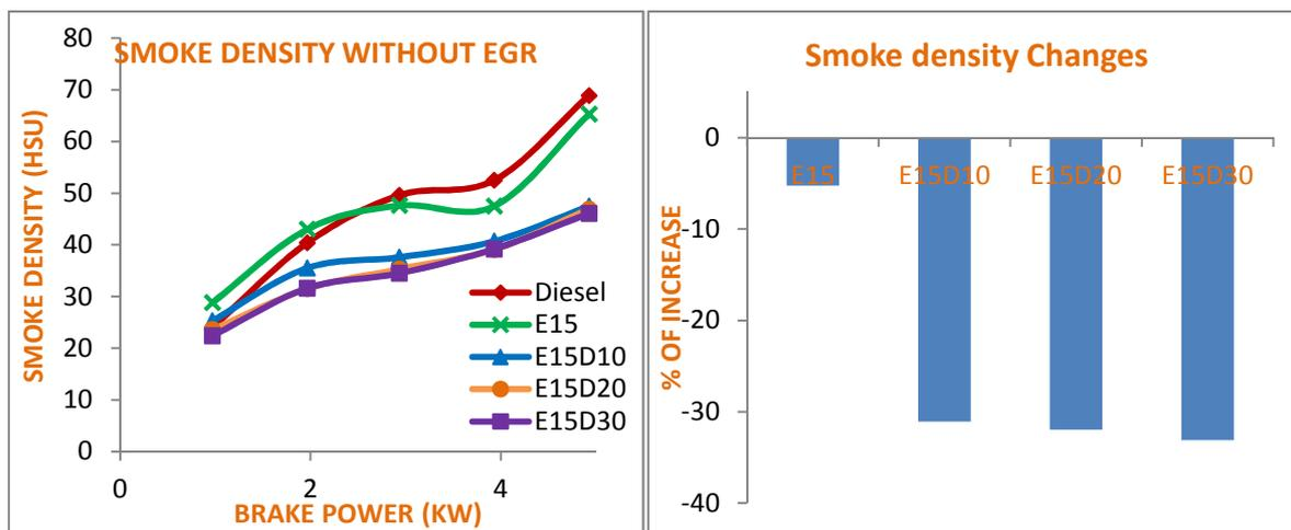
Fig 12: Brake power Vs Smoke Density.
