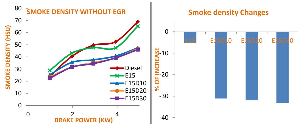
Fig 12: Brake power Vs Smoke Density.
