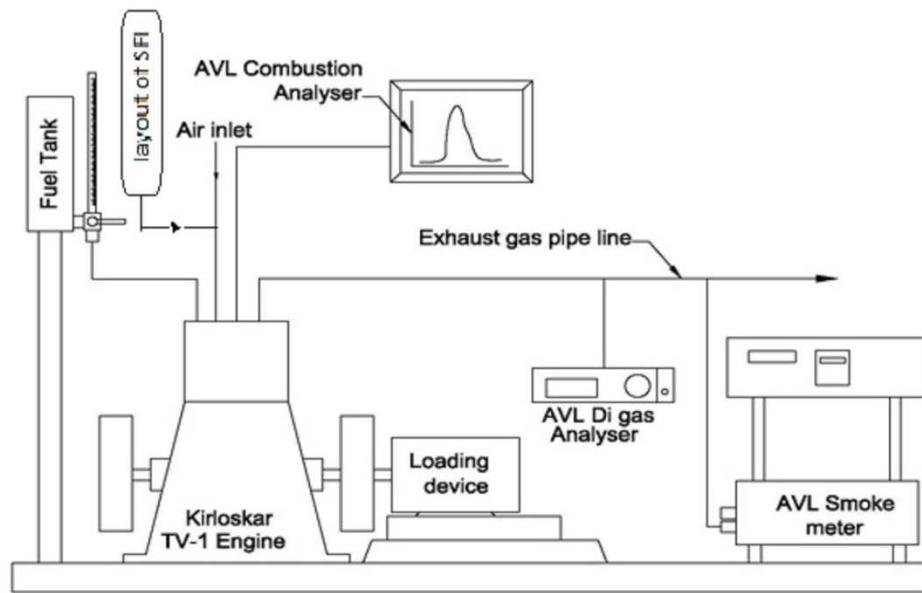
*Figure 1: Layout of Experimental Setup with Secondary Fuel injection (SFC).*
