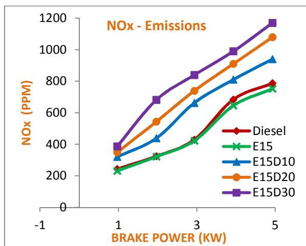
Fig 10: Brake power Vs NOx Emissions.
