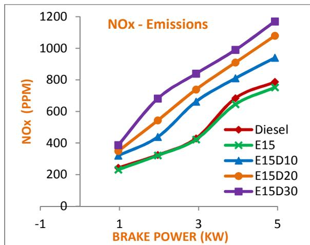
Fig 10: Brake power Vs NOx Emissions.
