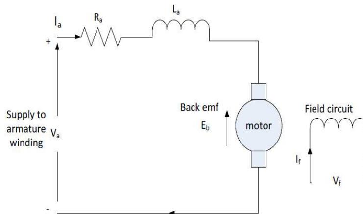
Figure 2. Separately Excited DC Motor Model
