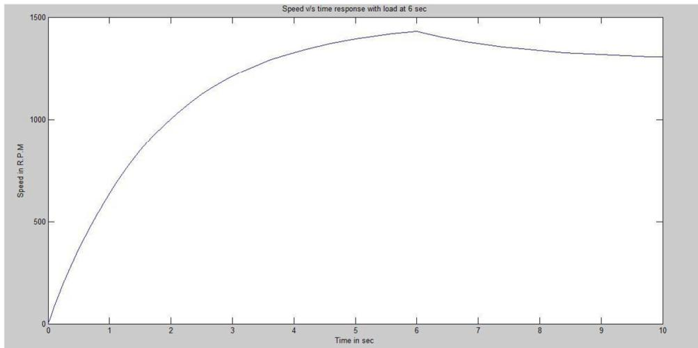
Figure 12. Speed Response of Chopper fed DC Motor using Fuzzy Logic Controller
