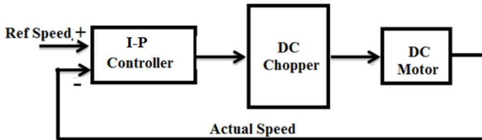
Figure 5. I-P Controller based Speed Control of Chopper fed DC Motor Comparative Analysis of Speed Response of Chopper Fed DC Motor using P-I and I-P Controller
