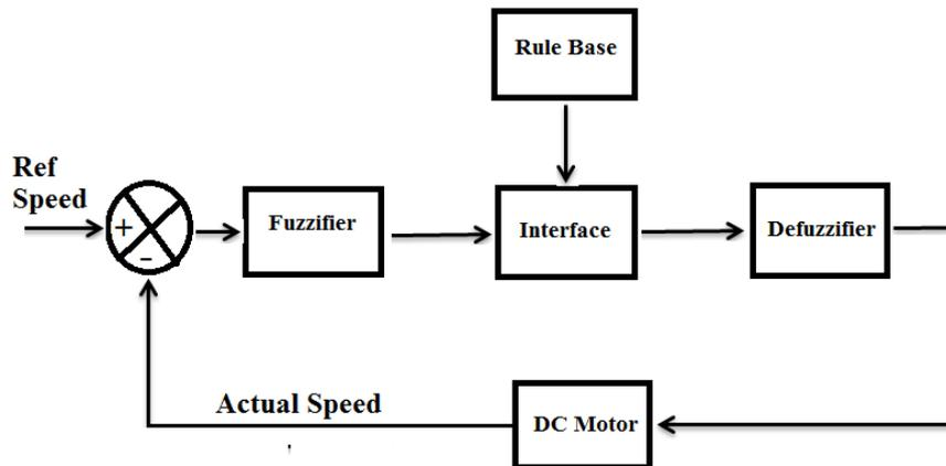
Figure 9. Block Diagram of Fuzzy Logic Controller
