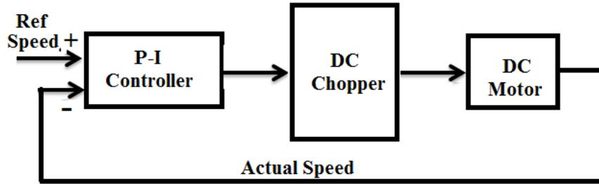
Figure 4. P-I Controller based Speed Control of Chopper fed DC Motor
