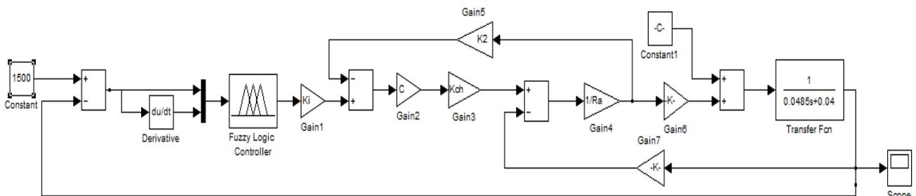
Figure 11. Simulink Model of FLC Control for Chopper fed DC Motor
