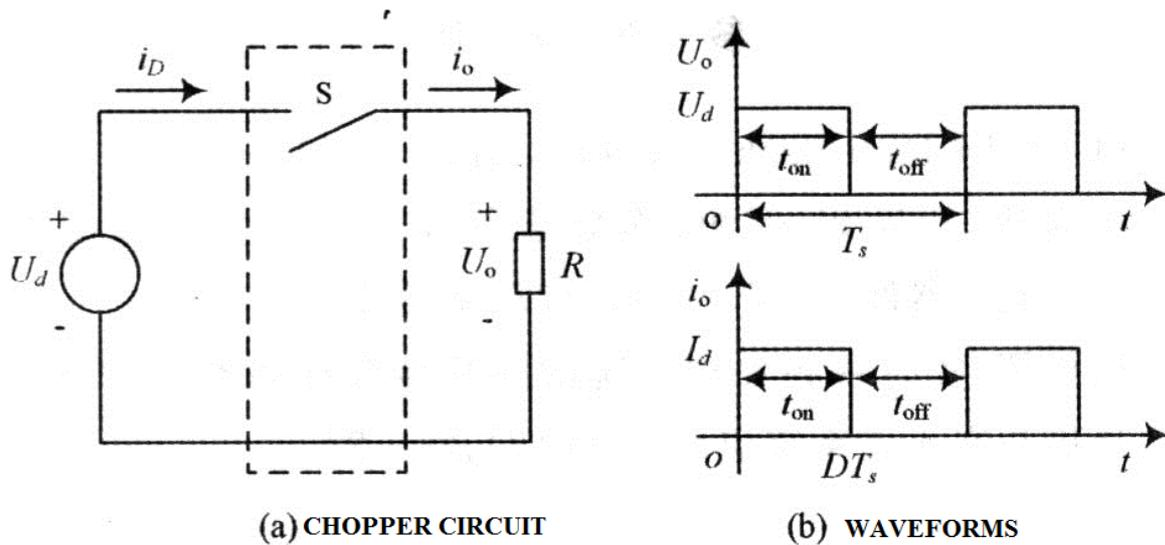
Figure 1. Chopper Circuit and its waveform
