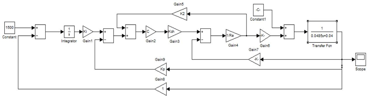
Figure 7. Simulink Model of I-P Control for Chopper fed DC Motor
