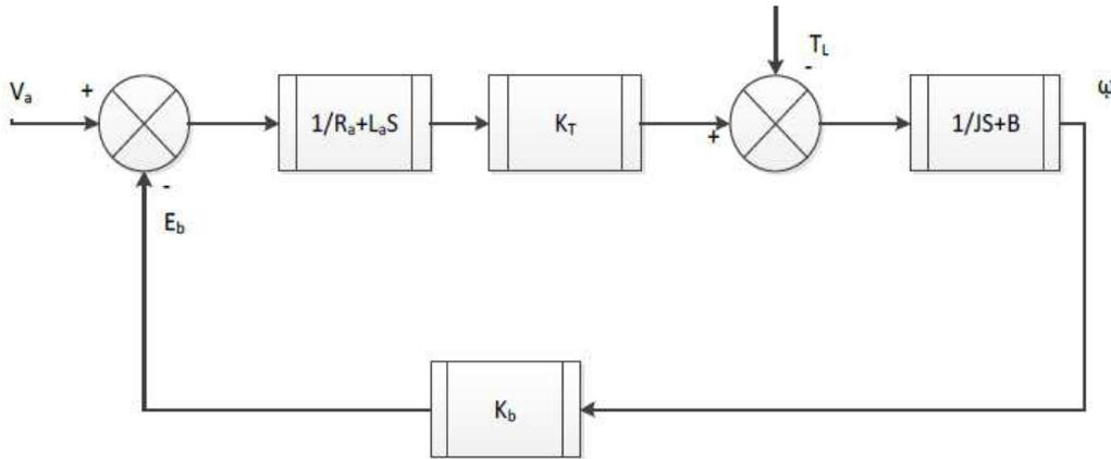
Figure 3. Block Model of Separately Excited DC Motor
