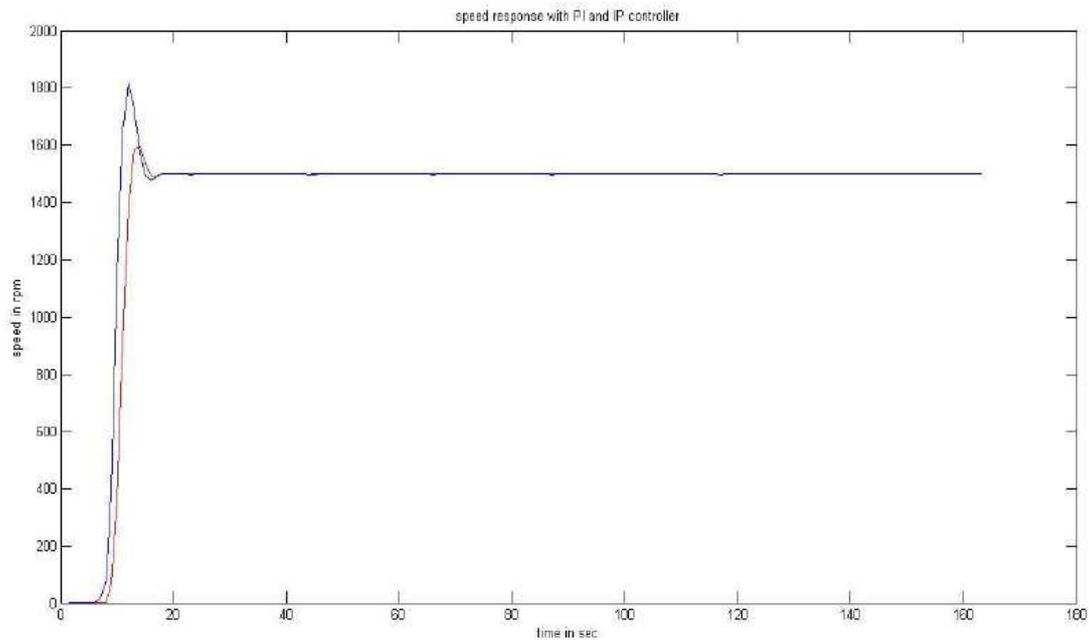
Figure 8. Comparison of Speed Response of Chopper fed DC Motor using P-I and I-P Controllers
