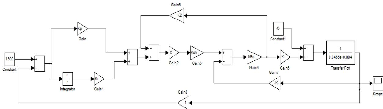
Figure 6. Simulink Model of P-I Control for Chopper fed DC Motor
