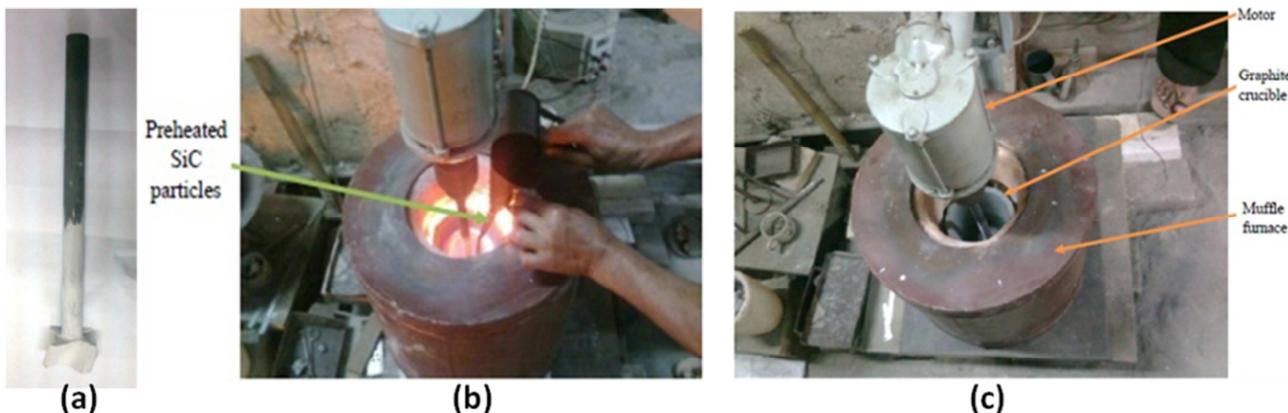
**Fig. 2 (a) Graphite stirrer, (b) Addition of SiC particles into the melt, (c) Stir casting setup**
