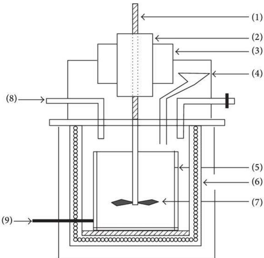
**Fig. 1: Schematic of stir casting setup. (1) Stirrer spindle, (2) sliding mechanism with impeller position control unit, (3) electric motor, (4) sprue, (5) crucible, (6) electric furnace, (7) impeller, (8) argon gas inlet, and (9) thermocouple; [14]**
