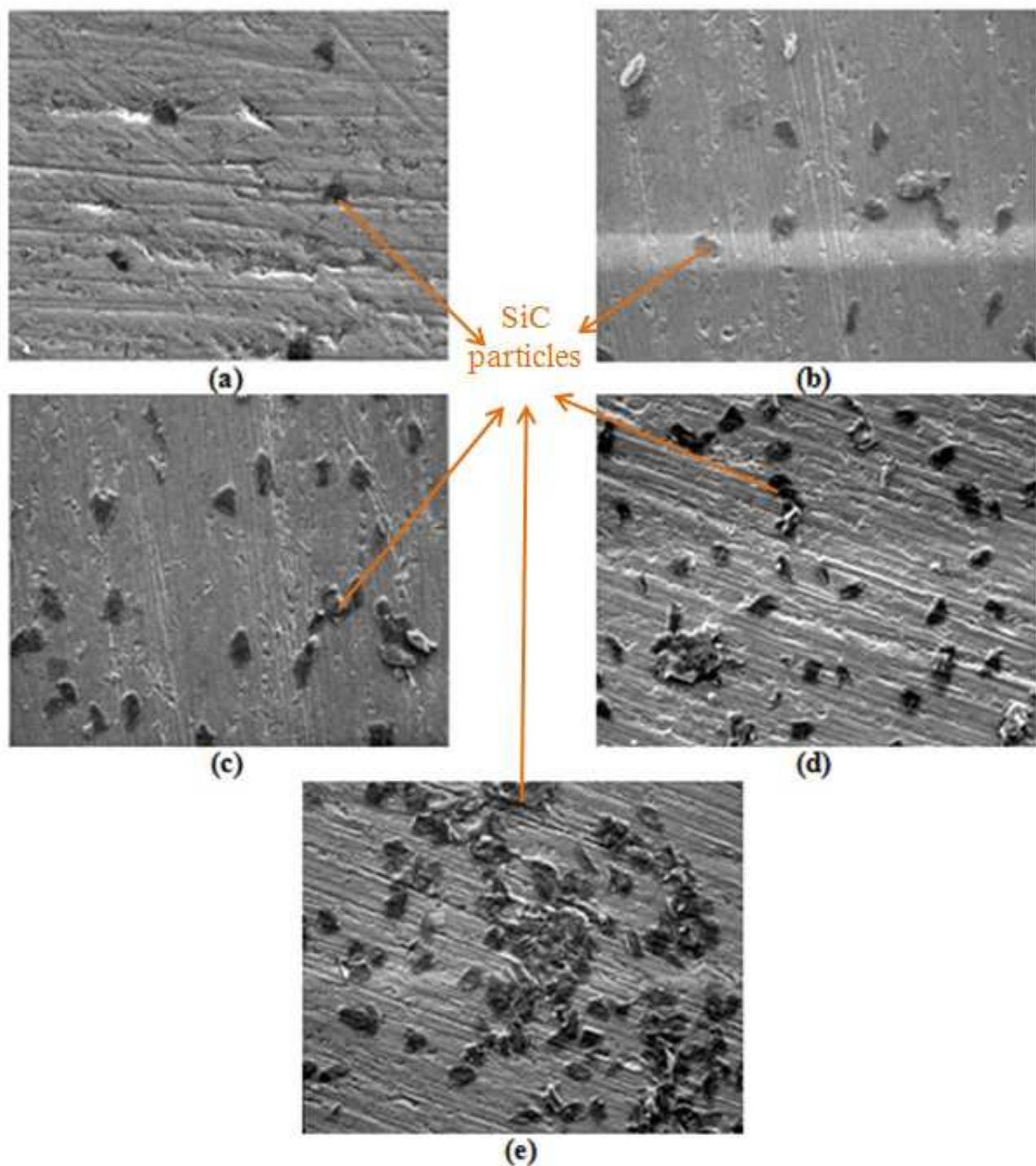
Fig. 3 Microstructure [Magnification : 250X] of composite with (a) 1 wt% SiC, (b) 3 wt% SiC, (c) 5 wt% SiC, (d) 7 wt% SiC and (e) 9 wt% SiC in the unetched condition.
