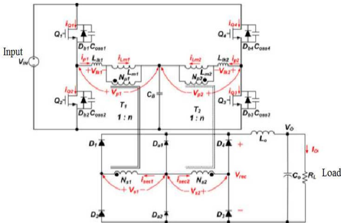
Fig. 3.2.1 Current and voltage indications in the proposed converter
