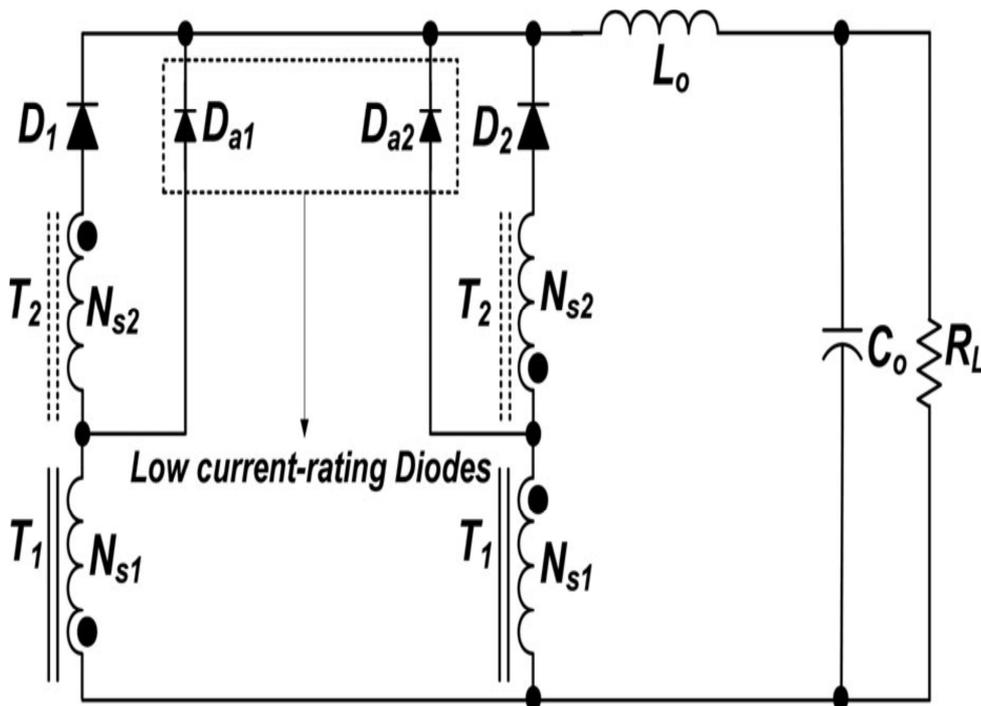
Fig. 5.4.1 Center-tap-type rectifier for the proposed converter design.
