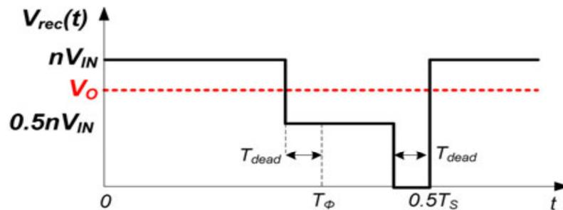
Fig. 5.1.1 Simplified design rectifier output waveform in the proposed converter
