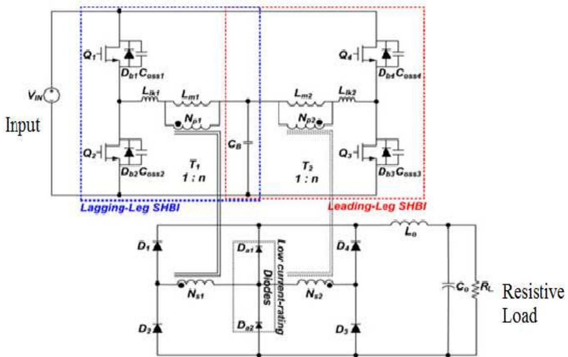
Fig. 3.1.1 Circuit diagram of the modified phase-shifted pulse width modulation converter
