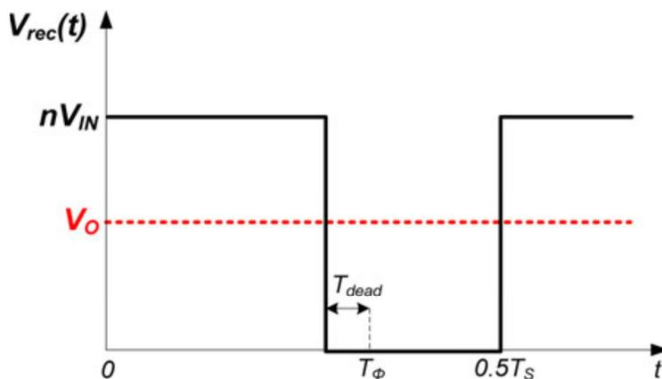
Fig. 5.1.2 Simplified design rectifier output in the existing converter with small leakage (or resonant) inductor
