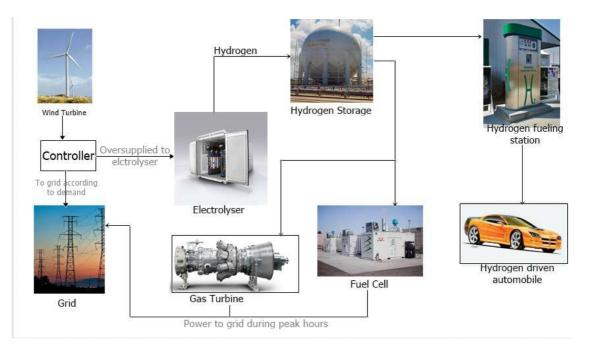
Fig. 5. A flow chart of Hydrogen production from wind and its utilization
