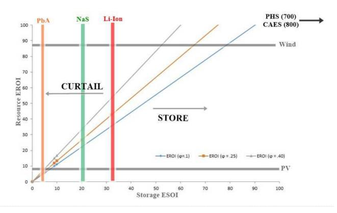
Fig. 4.Various combinations of resource EROI (y-axis) and storage ESOI (x-axis) for different value of curtailment or storage<br/>fraction (φ).
