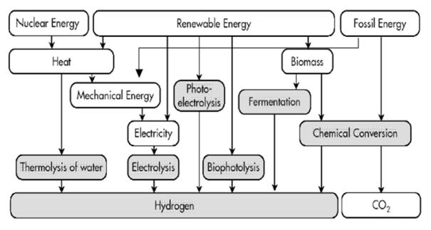
Fig. 1. Hydrogen production methods
