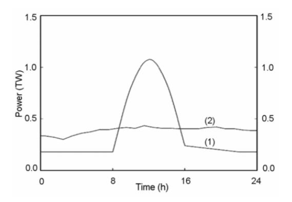
Fig. 2. Comparison of diurnal variation of production (curve 1) and demand (curve 2) over a typical sunny day.
