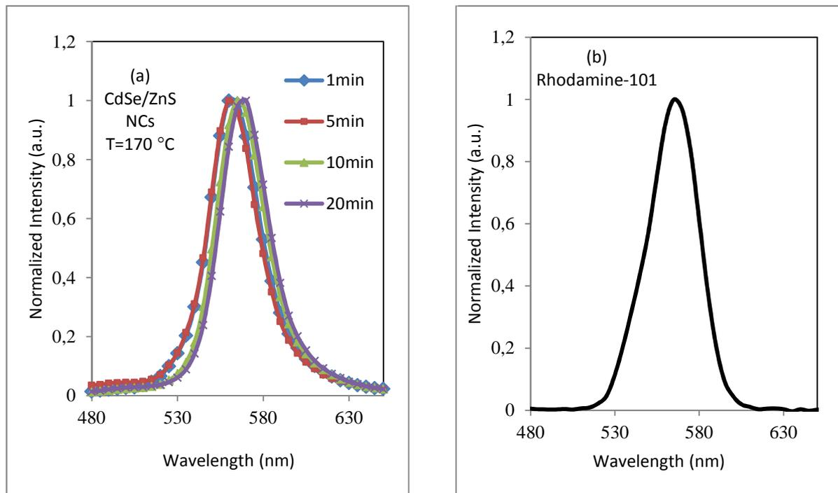
**Fig. 4. Normalized fluorescence emission spectra vs wavelength of (a) CdSe/ZnS Nanocrystals at 170<sup>o</sup> C for different times and (b) Rhodamine-101**
