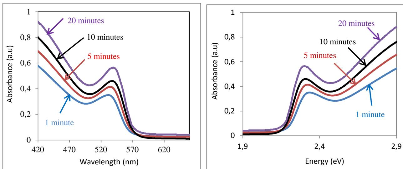
**Fig. 1. Absorbance spectra vs (a) wavelength and (b) energy of CdSe/ZnS Nanocrystals at 160° C for different times.**
