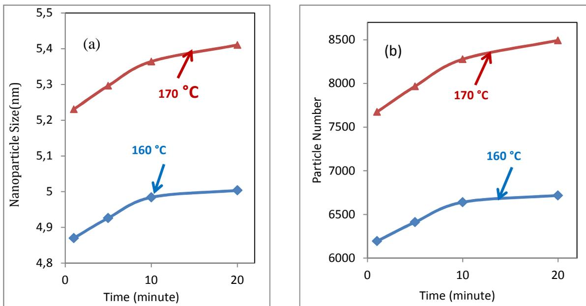
Fig. 2. (a) Nanoparticle size and (b) Particle number at the first peak absorption of CdSe/ZnS Nanocrystals for different times.
