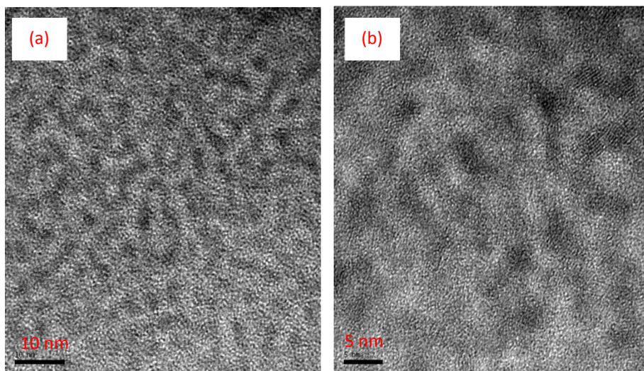
Fig. 3. TEM images of CdSe/ZnS nanocrystals at 20 minutes for (a) 160°C at 10 nm scale bar and (b) 170°C at 5 nm scale bar.
