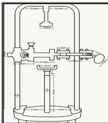
**Figure 1: Schematic diagram of the device with various dimensions**
