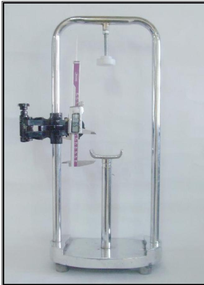
*Figure 3: Subject stabilizing device*
