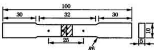
**Fig 5a. Smooth Tensile specimen details**
