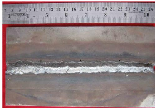
**Fig. 4. Fabricated joint using FCAW process**
