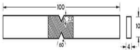
**Fig 5b. Notch Tensile specimen details**
