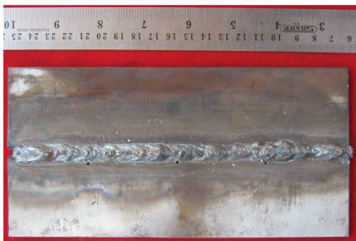
**Fig. 3. Fabricated joint using SMAW process**
