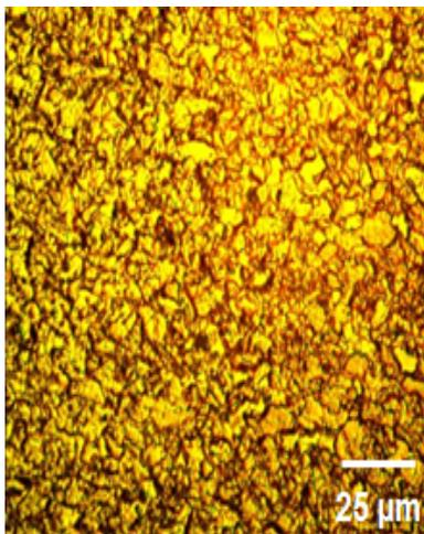
Fig.1c: Base metal microstructure
