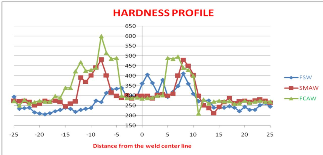
Fig. 6. Microhardness survey of all the Three Joints
