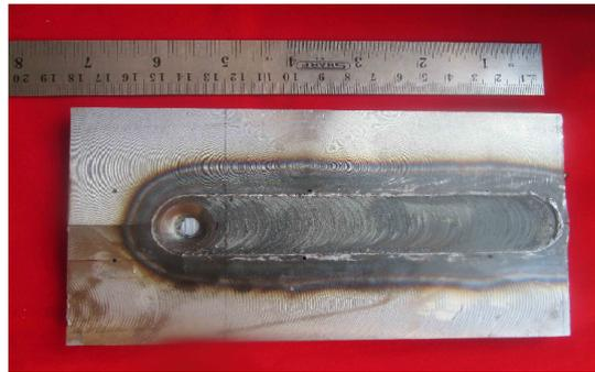
**Fig.2. Fabricated joint using FSW process**
