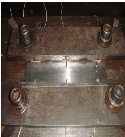
Fig.1e: Thermocouple location
