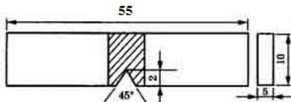
**Fig 5c. Impact specimen details**
