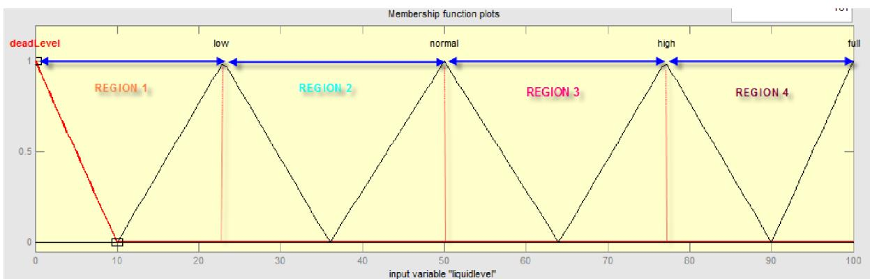
**Fig 3. Input liquid level membership function ranges**
