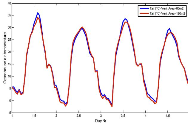
**Fig. 3.** The effect of ventilation area on greenhouse air temperature
