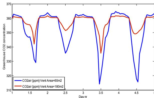
Fig. 5. The effect of ventilation area on greenhouse CO<sub>2</sub> concentration
