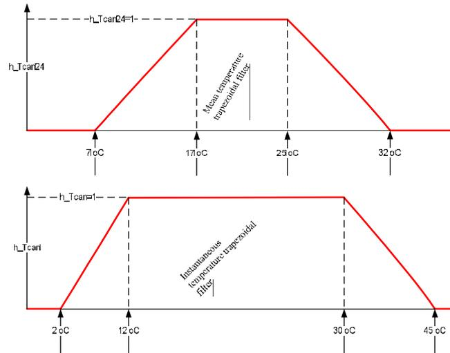
Fig. 1. Temperature growth inhibition factor computation method
