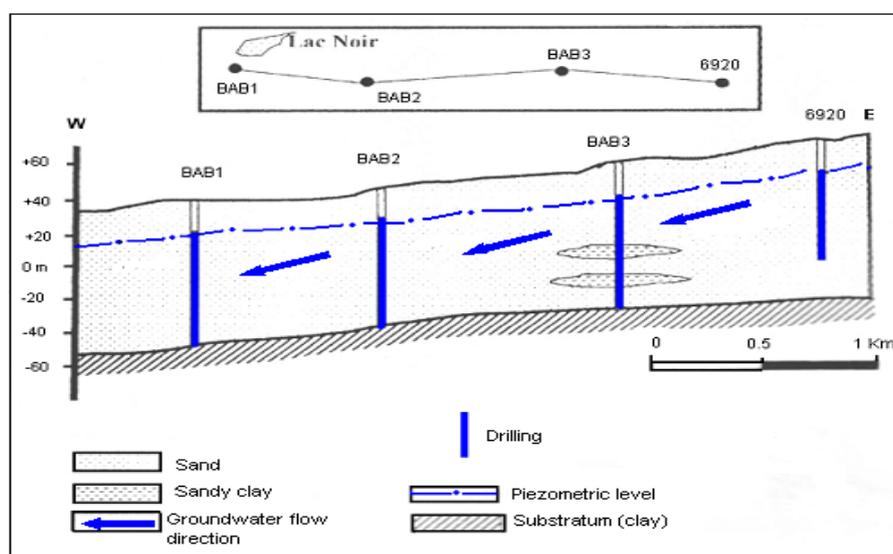
**Fig. 2. Hydrogeological section of the unconfined dune aquifer**
